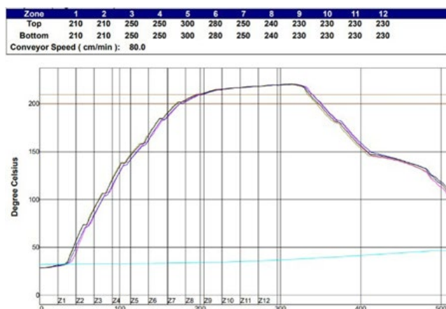
Figure 12. The reflow oven temperature profile for the experiments with mixed alloy powder solder paste.
