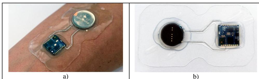
**Figure 6 : The final stretchable wireless sensor patch that was produced to test the manufacturing technologies in two versions a) with embedded battery and b) with an external charging interface.**
