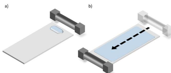
**Figure 2 : Schematic illustration of thin-film coating of silicone base layer. a) An appropriate volume of uncured liquid PDMS is deposited on the carrier in front of the bar applicator. b) The bar applicator is pulled over the uncured liquid PDMS, dispensed evenly on top of the carrier.**
