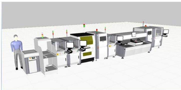
**Figure 1 : Concept of production line for stretchable electronics.**
