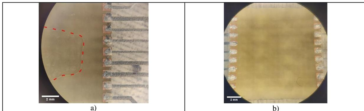
**Figure 5 : Micrographs of the backside of a rigid component mounted on liquid alloy circuitry and encapsulated. The Galinstan lines are in contact with the copper contact pads on the rigid component. The rigid components are encapsulated by a) high viscous PDMS only, where an air pocket is formed and marked by dotted line and b) completely underfilled by low-viscous PDMS and no air pocket is formed**
