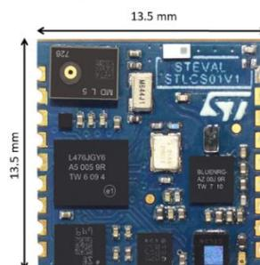
**Figure 4 :** The sensor module used in the demonstrator patch [10].
