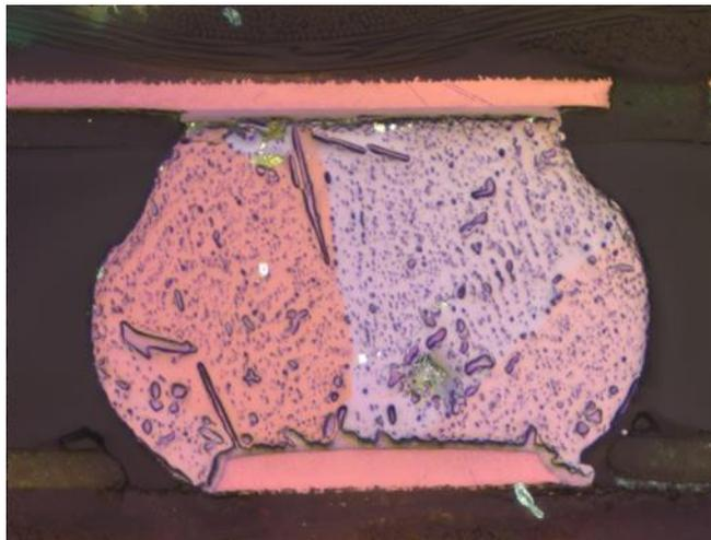
Fig. 11(b) Cross polarized image of cross section of a solder joint for SAC-Bi alloy
