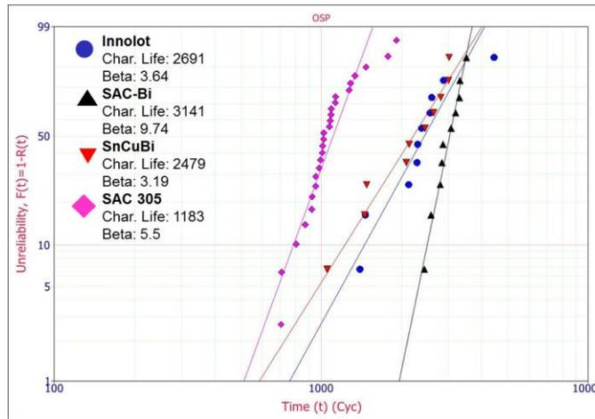
Fig. 8(a) Weibull analysis of different solder alloys with OSP surface finish
