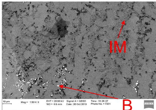
Fig. 2 Microstructure of non-aged Innolot alloy
