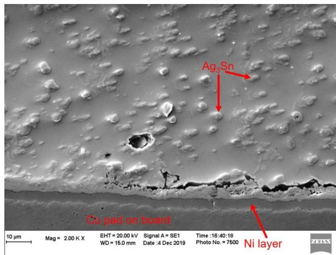
Fig. 10 Nickel layer for ENIG surface finish
