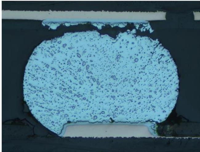
Fig. 11(a) Bright field image of cross section of a solder joint for Innolot alloy
