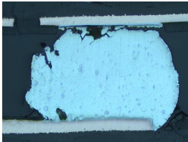
Fig. 11(c) Bright field image of cross section of a solder joint for SnCuBi alloy
