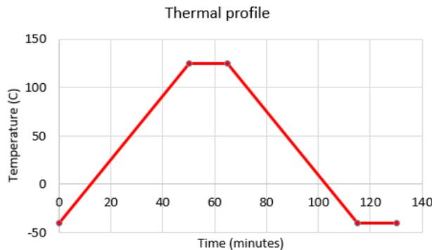
Fig. 5 Thermal cycling profile
