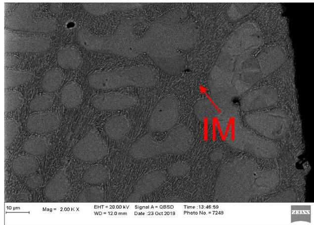
Fig. 1 Microstructure of non-aged SAC305 solder alloy
