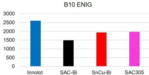
Fig. 6(c) B10 life for alloys with ENIG finish
