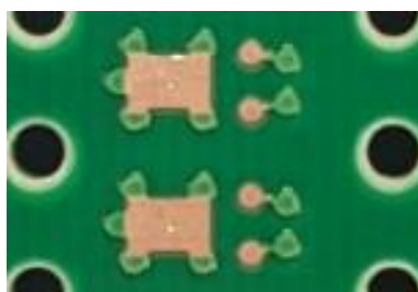
Figure 12. Via hole plugging coupon
