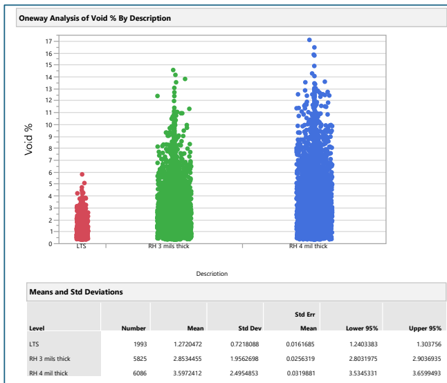
Figure 6. Impact of solder volume (modulated by stencil thickness) on Reverse Hybrid solder voids
