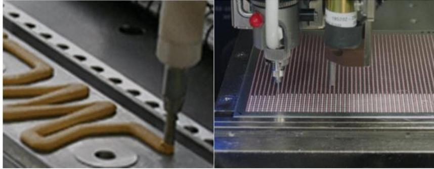
**Fig. 9 – Liquid dispensed bead/dots patterned for full coverage**
