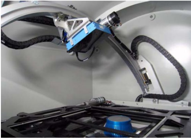
Figure 5. XRI system featuring FPD detector, the compact blue box mounted on the moving arc. X-ray source is on the bottom. Sample is position on a large tray that is placed on the frame. Sample tray is removed in this case in to show x-ray source. The detector moves full 360 degrees around the sample and can incline 70 degrees from the vertical.
