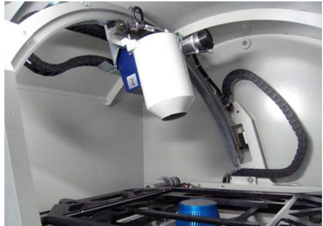
Figure 4. XRI system featuring II detector, the large white tube mounted on the moving arc. X-ray source is on the bottom. Sample is position on a large tray that is placed on the frame. Sample tray is removed in this case in to show x-ray source. The detector moves full 360 degrees around the sample and can incline 70 degrees from the vertical.
