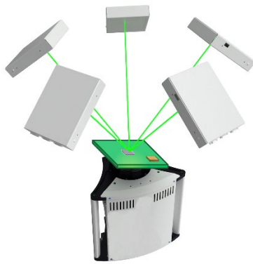
Figure 10. Working principle of planar CT (PCT). PCT keeps the sample flat and rotates the x-ray detector around it. X-ray source is on the bottom.
