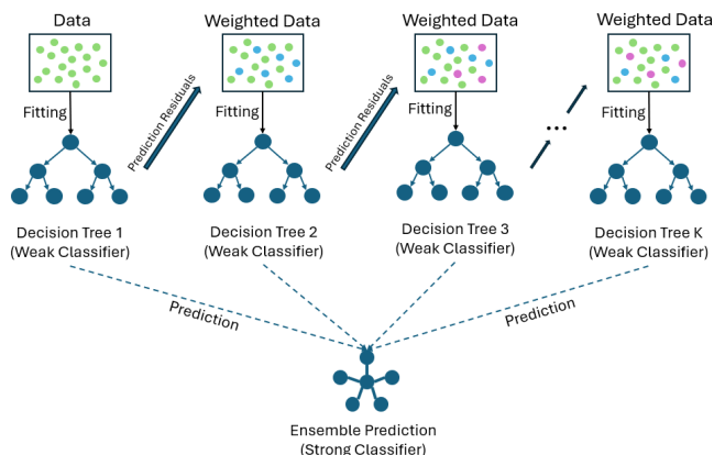
Figure 3: The architecture of a Gradient Boost Decision Tree model
