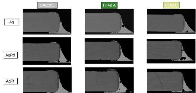
**Image 4.** SEM cross sections of 1206 chip capacitors of each solder/conductor combination after 1000 thermal cycles at -40°C to 150°C
