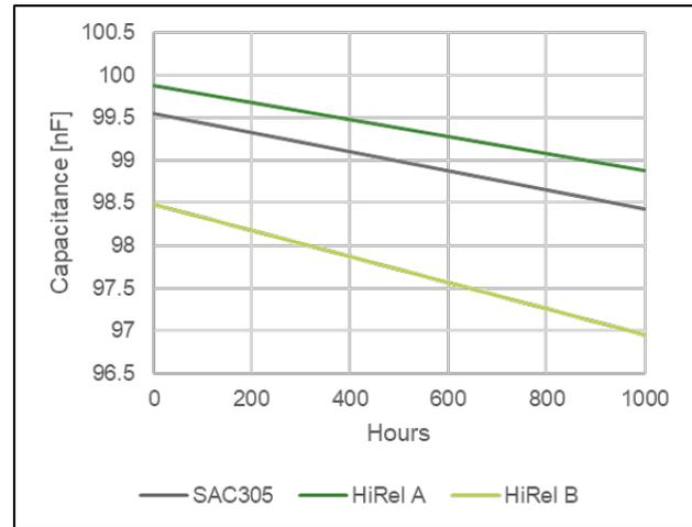
**Figure 17.** Capacitance trend of 1206 MLCCs in combination with Ag thick film conductor over 1000 thermal aging hours at 150°C
