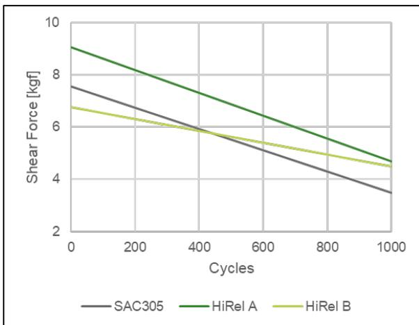
**Figure 7.** Shear force trend of 1206 MLCCs in combination with AgPd thick film conductor over 1000 thermal cycles at -40°C to 150°C
