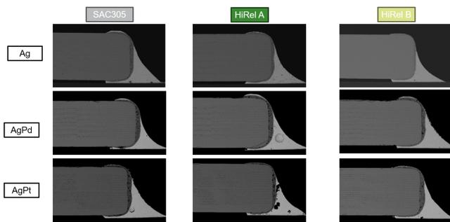
**Image 7.** SEM cross sections of 1206 MLCCs of each solder/conductor combination after 1000 hours at 150°C
