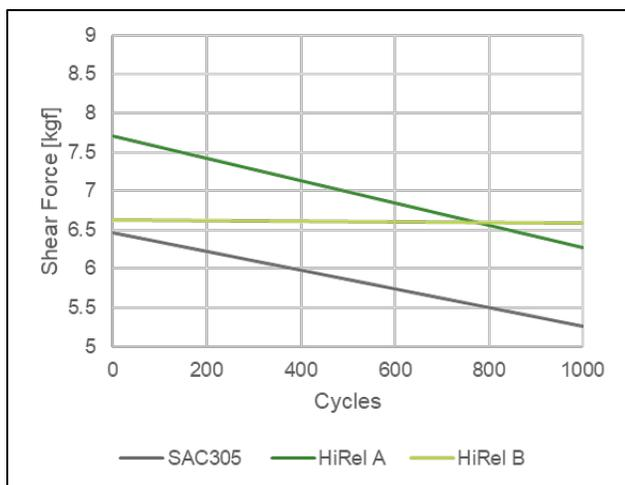
**Figure 4.** Shear force trend of 1206 chip resistors in combination with AgPd thick film conductor over 1000 thermal cycles at -40°C to 150°C
