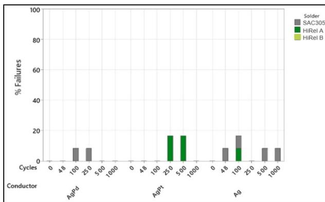
**Figure 11.** Percent of failed 0402 MLCCs that changed in capacitance of >10% after 1000 cycles at -40°C to 150°C
