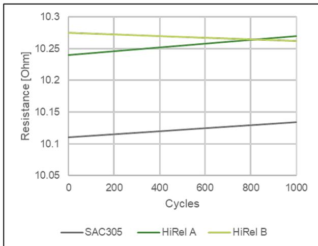
**Figure 3.** Resistance trend of 1206 chip resistors in combination with AgPd thick film conductor over 1000 thermal cycles at -40° to 150°C
