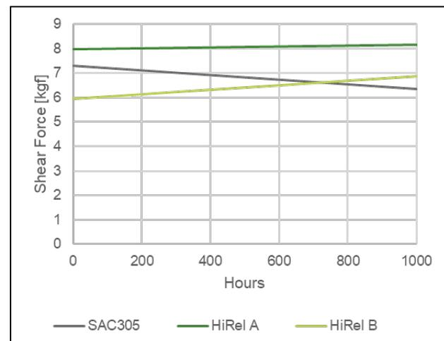
**Figure 18.** Shear trend of 1206 MLCCs in combination with Ag thick film conductor over 1000 thermal aging hours at 150°C
