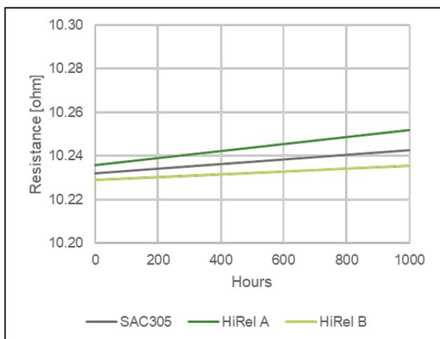
**Figure 12.** Resistance trend of 1206 chip resistors in combination with AgPd thick film conductor over 1000 thermal aging hours at 150°C
