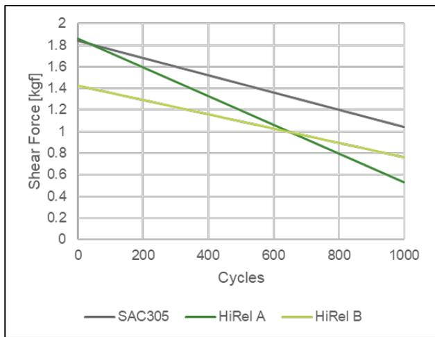
**Figure 10.** Shear force trend of 0402 MLCCs in combination with Ag thick film conductor over 1000 thermal cycles at -40°C to 150°C
