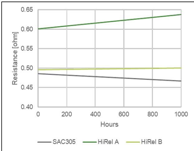
**Figure 15.** Resistance trend of 0402 chip resistors in combination with AgPt thick film conductor over 1000 thermal aging hours at 150°C
