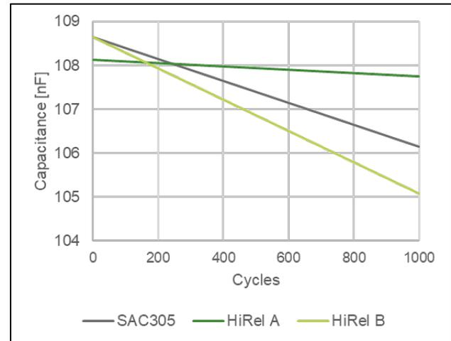
**Figure 9.** Capacitance trend of 0402 MLCCs in combination with AgPd thick film conductor over 1000 thermal cycles at -40°C to 150°C
