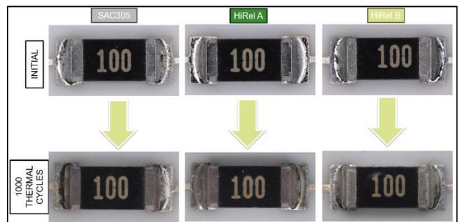
**Image 5.** 1206 chip resistors of each solder type before and after thermal aging 1000 hours at 150°C
