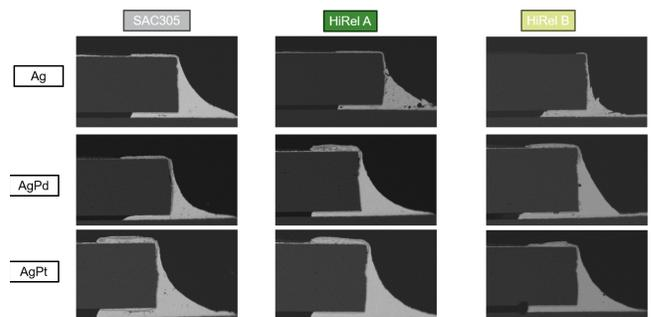
**Image 6.** SEM cross sections of 1206 chip resistors of each solder/conductor combination after 1000 hours at 150°C
