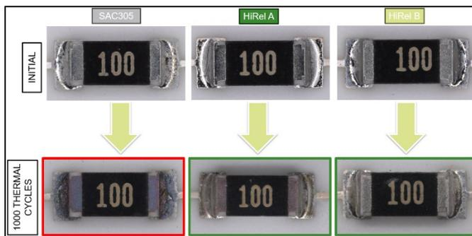
**Image 2.** 1206 chip resistors with each solder type, each
