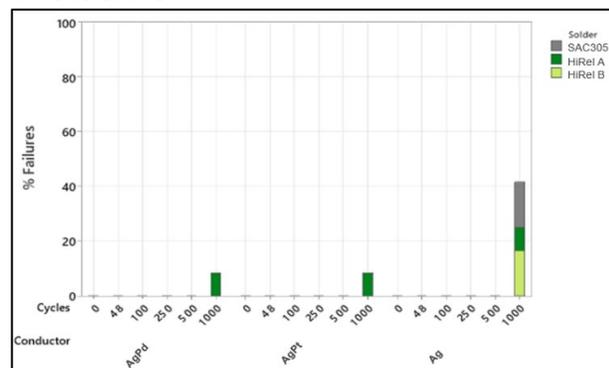
**Figure 8.** Percent of failed 1206 MLCCs that changed in capacitance of >10% after 1000 cycles at -40°C to 150°C
