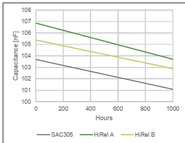
**Figure 19.** Capacitance trend of 0402 MLCCs in combination with AgPd thick film conductor over 1000 thermal aging hours at 150°C
