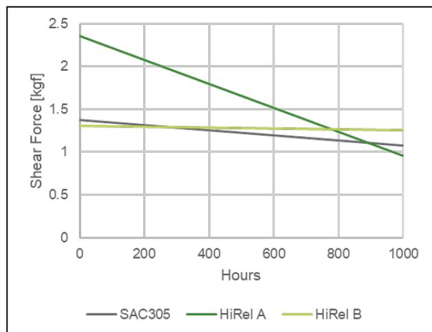
**Figure 20.** Shear trend of 0402 MLCCs in combination with AgPd thick film conductor over 1000 thermal aging hours at 150°C
