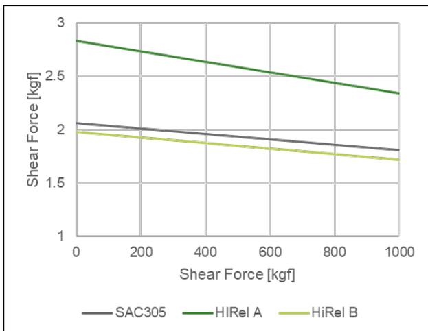
**Figure 16.** Shear trend of 0402 chip resistors in combination with AgPt thick film conductor over 1000 thermal aging hours at 150°C
