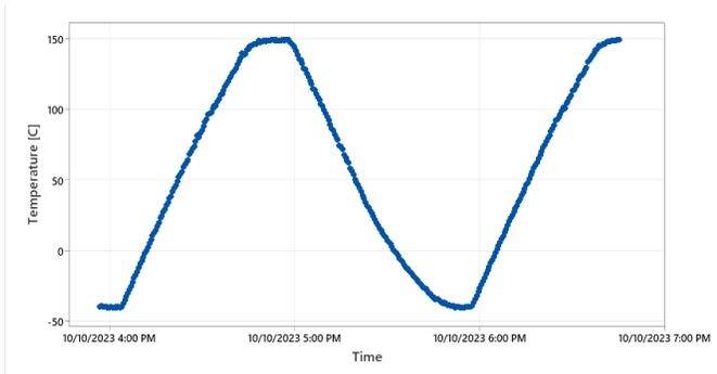
**Figure 2.** Thermal cycling profile
