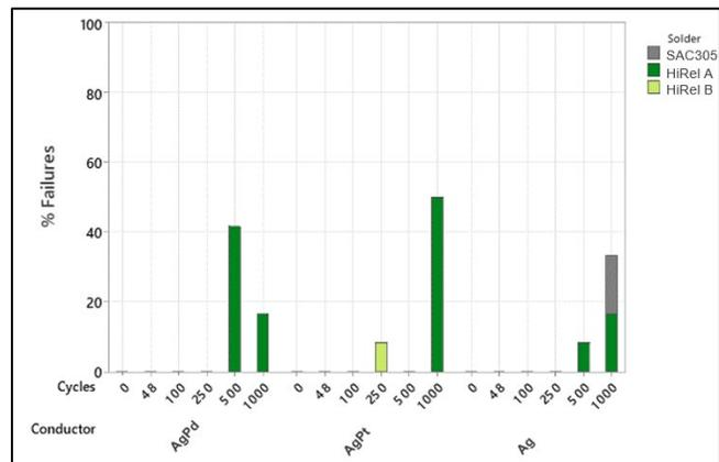
**Figure 5.** Percent of failed 0402 chip resistors with a percent change in resistance of >10% after 1000 cycles at -40°C to 150°C
