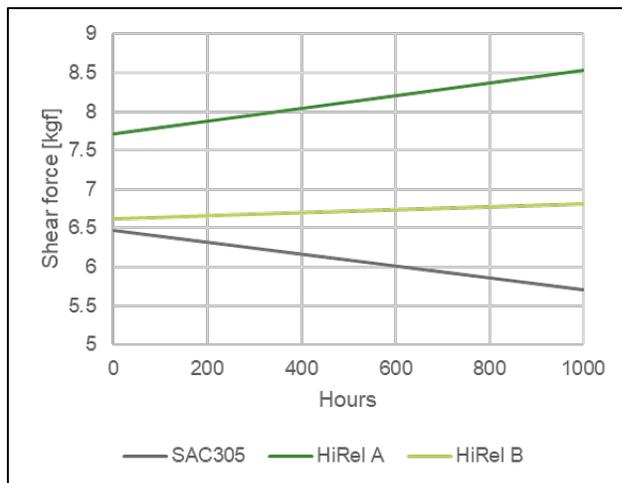
**Figure 13.** Shear trend of 1206 chip resistors in combination with AgPd thick film conductor over 1000 thermal aging hours at 150°C
