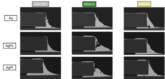
**Image 3.** SEM cross sections of 1206 chip resistors of each solder/conductor combination after 1000 thermal cycles at -40°C to 150°C
