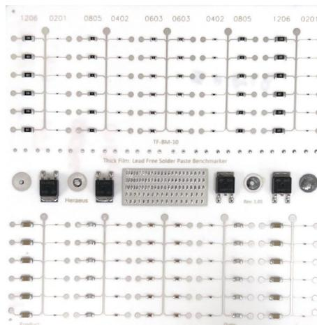
**Image 1.** Example of control test vehicles after solder reflow.
