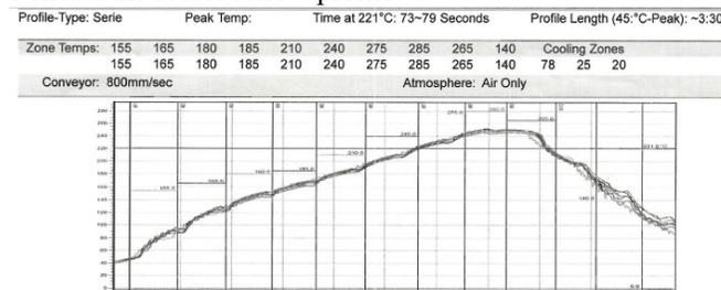
**Figure 1.** Solder reflow profile
