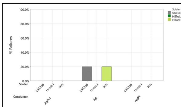
**Figure 14.** Percent of failed 0402 chip resistors that changed in resistance of >10% after 1000 hours of thermal aging at 150°C
