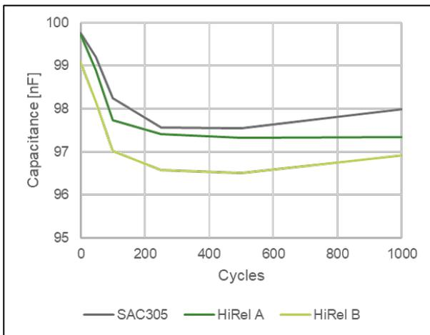
**Figure 6.** Capacitance trend of 1206 MLCCs in combination with AgPd thick film conductor over 1000 thermal cycles at -40°C to 150°C
