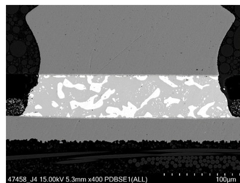
Figure 8. System A, power FET switch pin post-2.5 years daily corporate use
