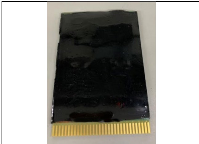
Figure 10. Encapsulation Resin Image after Condensation IR test
