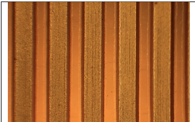
Figure 7. Image of Bare PCB – Solvent Based Coating after SIR
