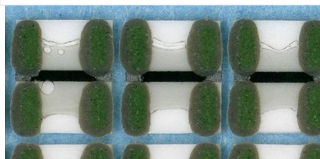
Figure 26: Glass Test Board with 200 Chips for evaluating cleaning after 10 minutes
