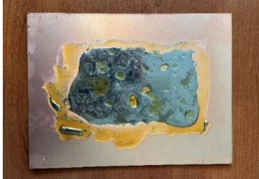
Figure 9: Flux Residue Post Reflow
