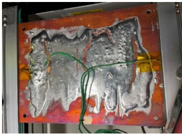
Figure 8: Solder Paste Loading board for profiling
