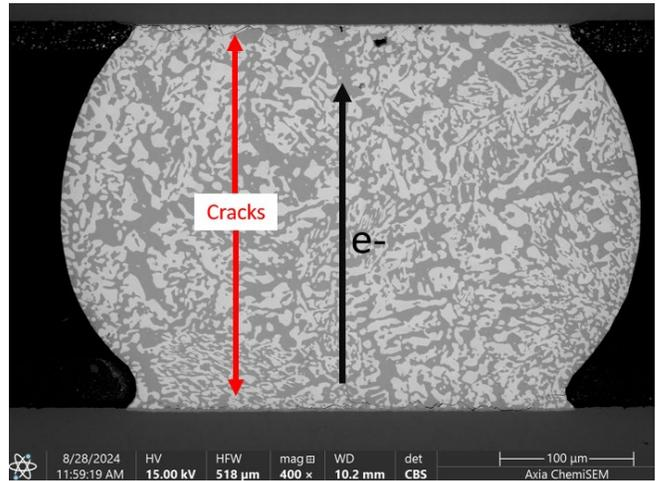
**Figure 13.** Cross-section of corner most solder joint subjected to drop testing after 120 days of 75°C 0.50A stressing. Bismuth accumulation at the anode is apparent. Note that the primary crack is located at the joint cathode, near the PCB.
