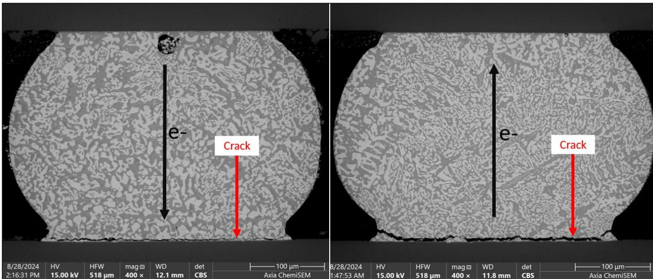
**Figure 16.** Cross-section of corner most solder joints subjected to drop testing after 30 days of 75°C 2.27A stressing. Note that the cracks are located at the joint anode (left) and joint cathode (right) near the PCB.
