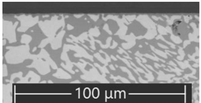
**Figure 15.** Cross-section showing solder joint anode region after 120 days of 75°C 0.80A stressing. Careful inspection indicates that bismuth has accumulated in this region.
