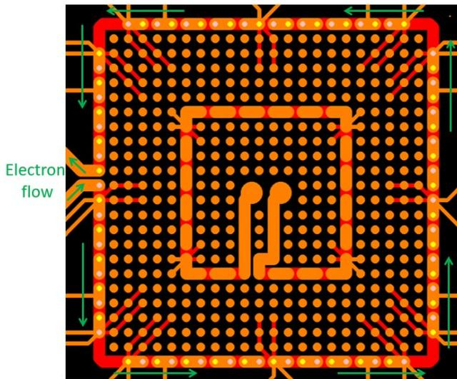
**Figure 6.** BGA/PCB electrical map. Orange indicates PCB copper features, Red indicates BGA features. Yellow indicates electron flow from BGA toward PCB (down), grey indicates electron flow from PCB toward BGA (up). Only perimeter joints were current stressed.
