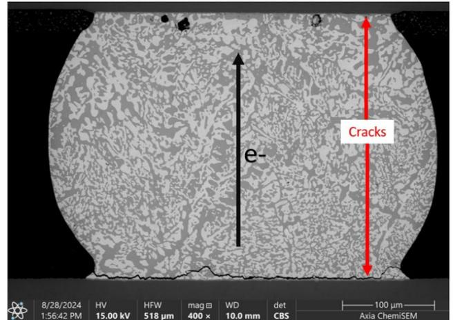
**Figure 14.** Cross-section of corner most solder joint subjected to drop testing after 120 days of 75°C 0.80A stressing. Note that the primary crack is located at the joint cathode, near the PCB.
