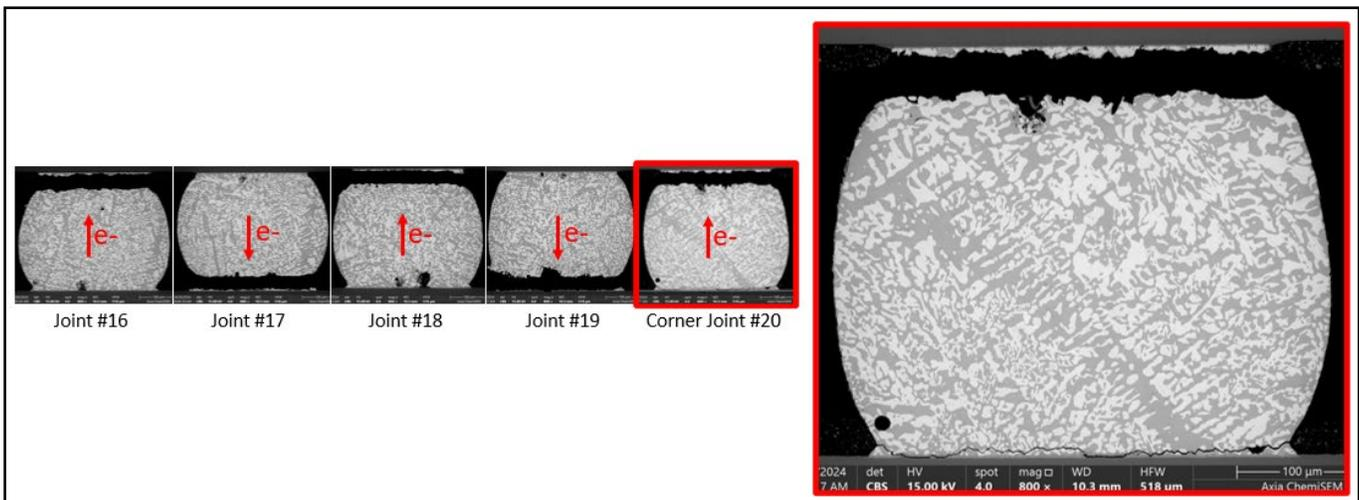
**Figure 19.** Cross-sectioned joints from 85°C 0.80A 75-day population showing complete cracking at the anode side of five sequential solder joints.
