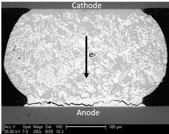
**Figure 5.** Scanning electron micrograph showing SnBiSbNi BGA solder joint stressed at 4.2A and 100°C for 120 hours and drop tested. Bismuth accumulation at the anode side and lack of bismuth near the cathode side are apparent [3].
