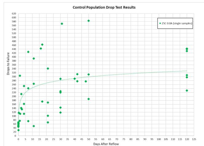
Figure 9. Scatterplot showing drop test results for Control Population as a function of time after assembly. Data previously published in [4] with additional data provided for 120 days.
