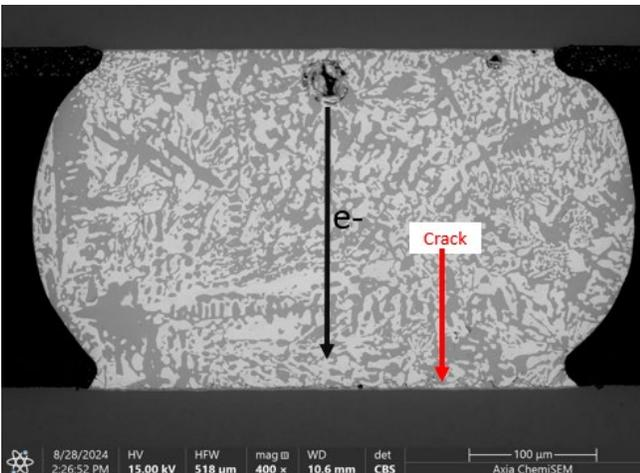
**Figure 12.** Cross-section of corner most solder joint subjected to drop testing after 120 days of 75°C 0.25A stressing. Note that the primary crack is located at the joint anode, near the PCB.
