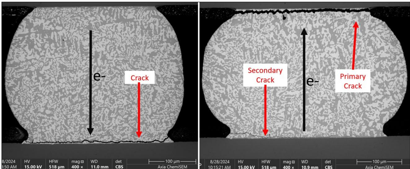
**Figure 21.** Cross-sectioned joints from 100°C 2.27A 20-day population showing corner joints with complete cracking at their anodes.
