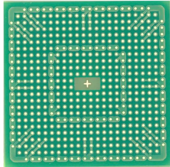
**Figure 2.** Image of BGA556 solder ball side prior to ball attachment.
