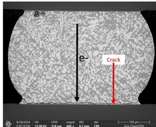
**Figure 18.** Cross-section of corner-most solder joint subjected to drop testing after 120 days of 85°C 0.50A stressing. Note that the primary crack is located at the joint anode near the PCB. All samples subjected to 85°C 0.50A for 120 days failed at “anode down” solder joint positions indicating a strong influence of bismuth migration on drop test performance.
