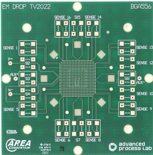
**Figure 1.** Image of Test Board Side A with BGA556 footprint.
