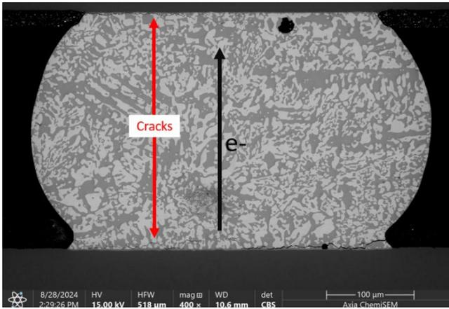
**Figure 11.** Cross-section of corner most solder joint subjected to drop testing after 120 days of 75°C 0.25A stressing. Note that the primary crack is located at the joint cathode, near the PCB.
