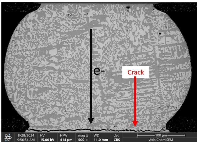
**Figure 22.** Cross-sectioned joint from 100°C 1.20A 30-day population showing complete cracking at the anode side. Populations which were temperature / current stressed at a mild service-like condition of 0.25A with a solder joint temperature of 75°C did not show obvious bismuth accumulation through 120 days. These samples failed due to solder fracturing near the PCB side of the corner-most joints regardless of anode and cathode position, which was similar to the Control population behavior.
