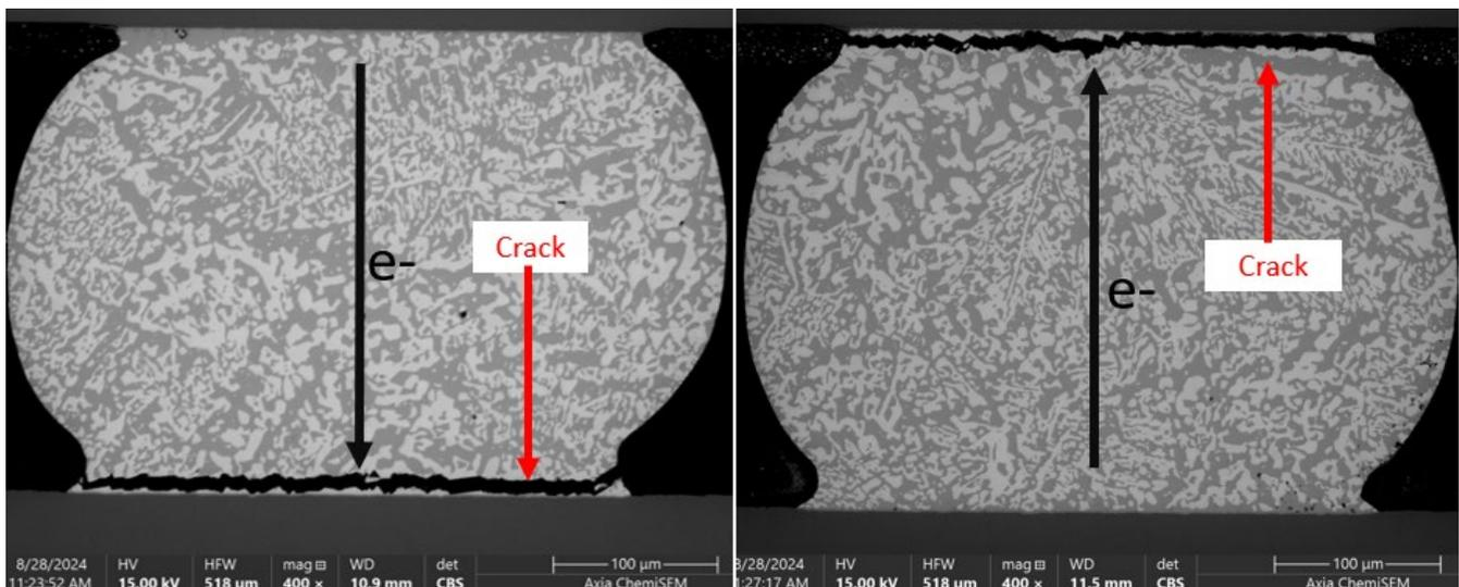
**Figure 20.** Cross-sectioned joints from 85°C 2.84A 45-day population showing complete cracking at the anode side of the solder joints. The left image shows a thin, solid layer of bismuth has formed at the anode. The right image shows a thin, incomplete layer of bismuth has formed at the anode.
