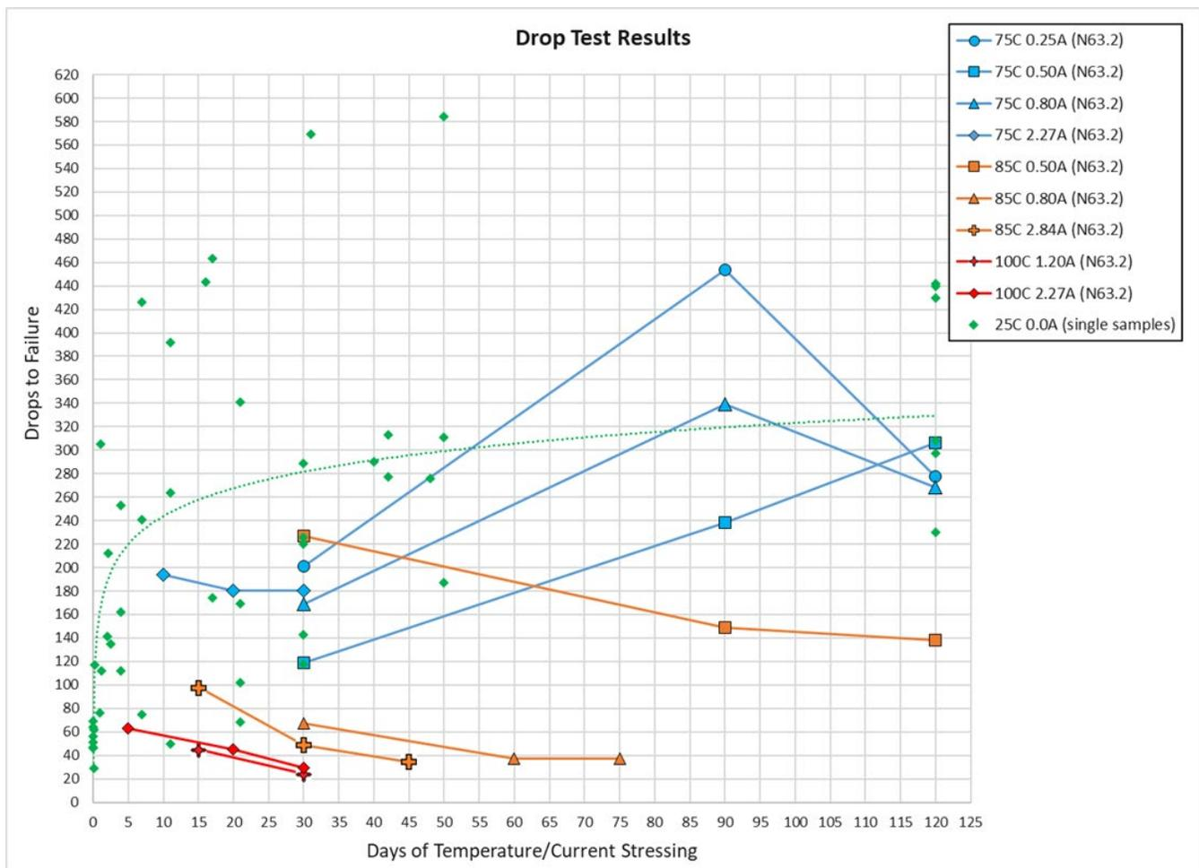
**Figure 10.** Characteristic Lifetimes vs. Stress Duration Overlaid with Control Data. Blue indicates solder joint temperatures of 75°C; Orange indicates solder joint temperatures of 85°C; Red indicates solder joint temperatures of 100°C; Green indicates Control samples (i.e. no current stress conditioning; ambient storage)
