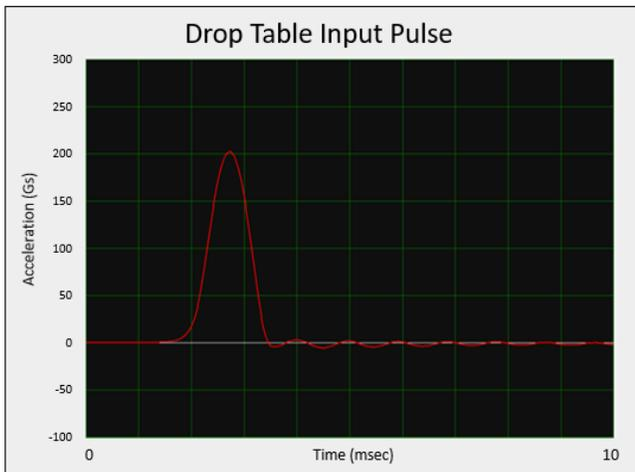
Figure 8. Example drop table input pulse.
