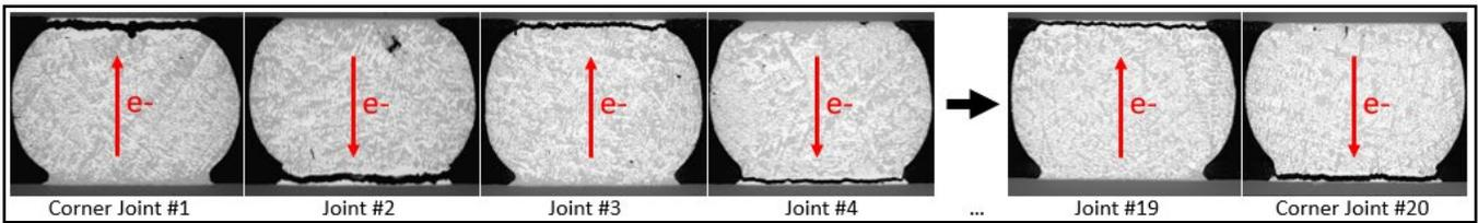
**Figure 4.** Scanning electron micrographs showing SnBiSbNi BGA solder joints stressed at 4.2A and 100°C for 120 hours and drop tested. All joints in the field of view failed at the anode side where bismuth accumulation had occurred [3].
