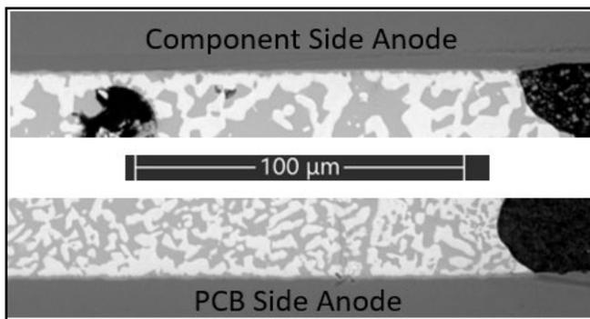
**Figure 17.** Comparison between component and PCB side anodes from 30 day 75°C 2.27A population. Bismuth density along the anodes was significantly greater than bismuth density at the cathodes.
