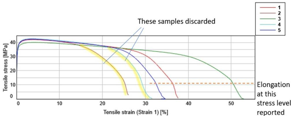
**Figure 6.** Typical tensile stress strain plots showing criteria for selecting 3 results out of 5 repeats and method of defining elongation.
