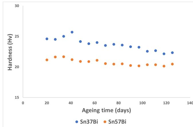
**Figure 16.** Hardness of representative tin-bismuth alloys as function of ageing time at room temperature
