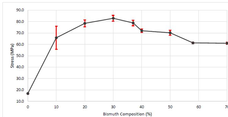
**Figure 14.** Ultimate tensile strength at a strain rate of  $0.00079 \text{ s}^{-1}$  of tin-bismuth alloys as a function of bismuth content.
