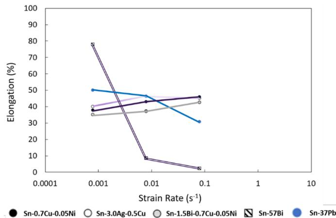
**Figure 9.** Elongation as a function of strain rate [17].
