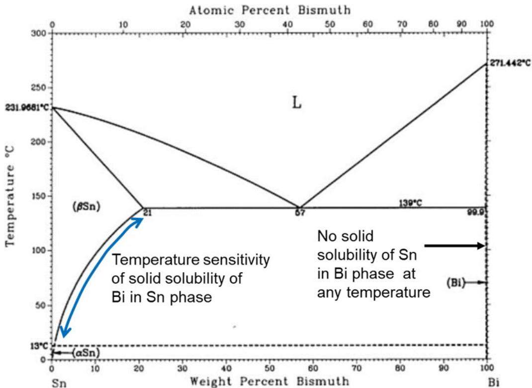
**Figure 1.** Tin-bismuth phase diagram highlighting the temperature sensitivity of the solid solubility of bismuth in tin [6]
