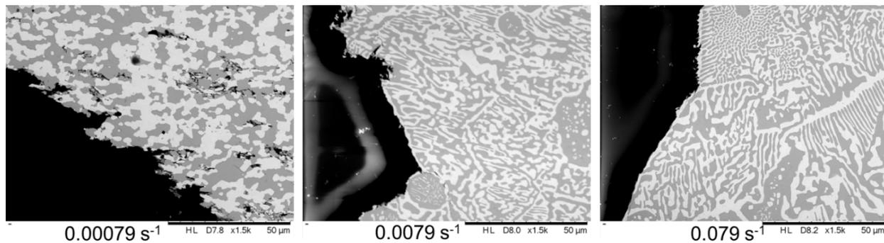
**Figure 11.** Microstructure close to the fracture of Sn-57Bi at the indicated strain rates.
