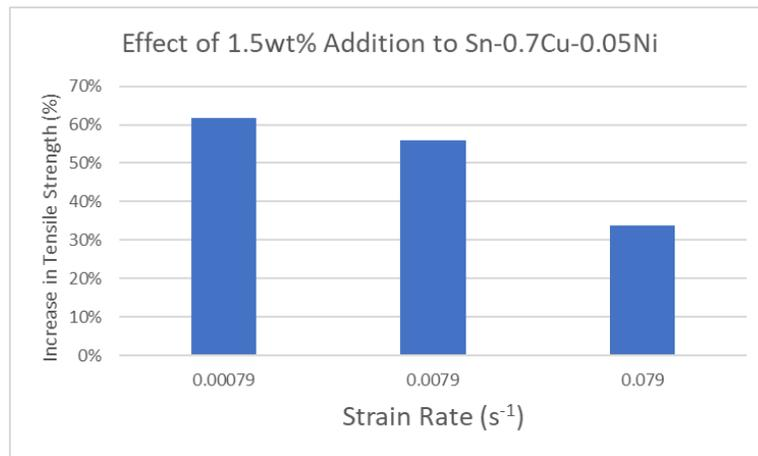
**Figure 17.** Effect of 1.5Bi addition SN-0.7Cu-0.05Ni on tensile strength
