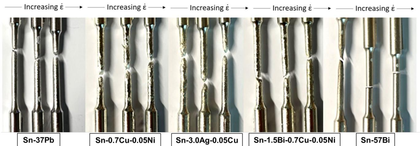
**Figure 10.** Character of strain and fracture as a function of alloy and strain rate
