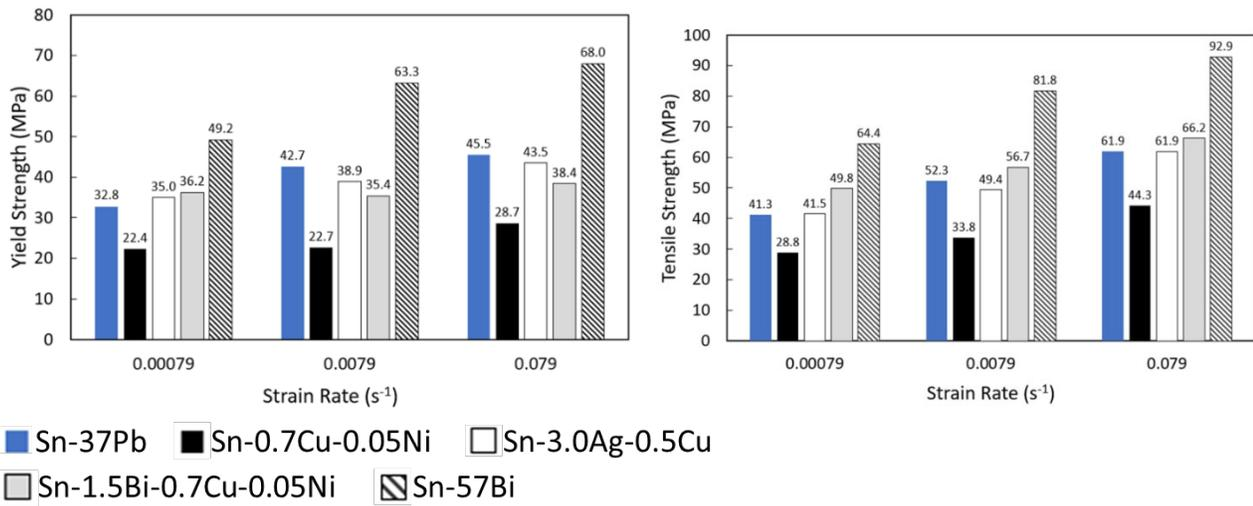
**Figure 7.** Yield Stress (0.2% Proof Stress) and Ultimate Tensile Strength as a function of strain rate.[17].
