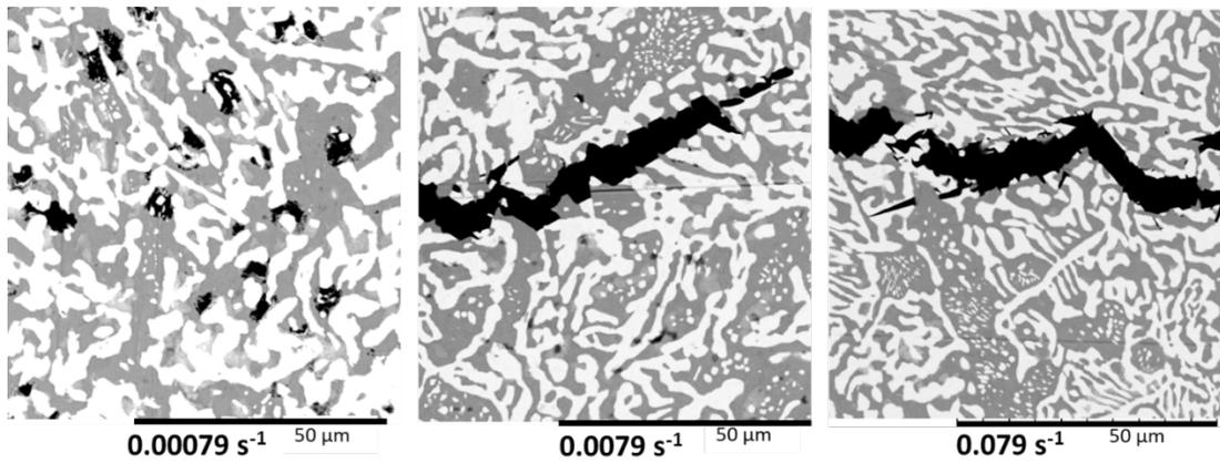
**Figure 13.** Damage initiation in the microstructure of Sn-57Bi before fracture.
