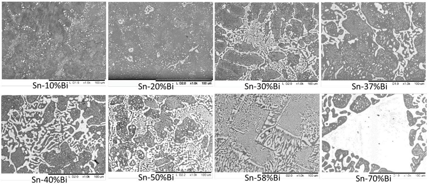
Figure 5. Microstructure of tin-bismuth alloys tested
