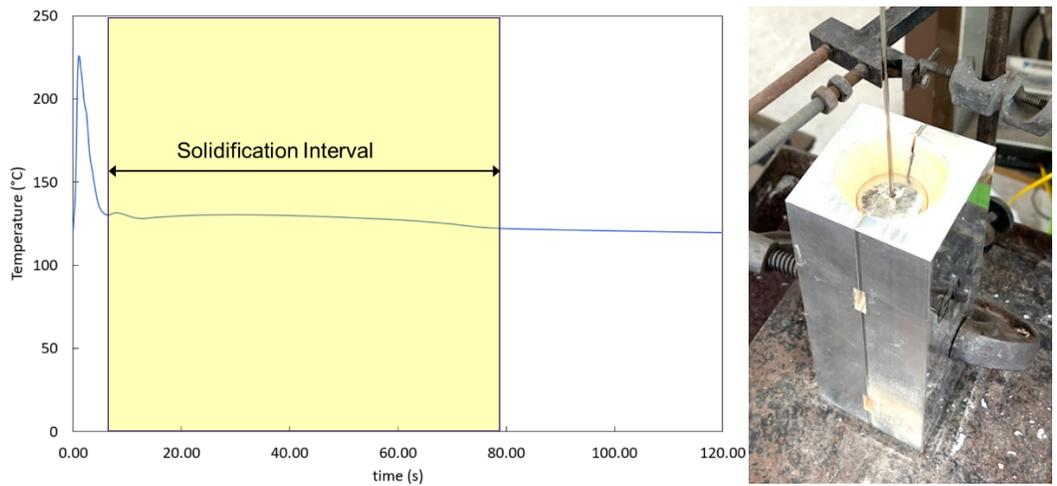
**Figure 3.** Typical cooling curve for cast test piece and thermocouple monitoring
