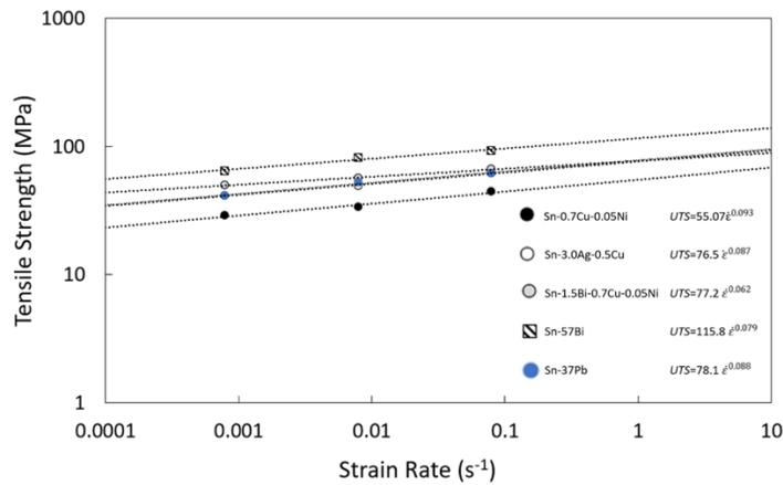
**Figure 8.** Logarithmic plot of Ultimate tensile strength as a function of strain rate [17].
