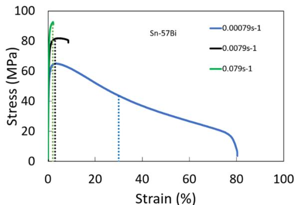
**Figure 12.** Tensile tests of Sn-57Bi stopped before failure. Solid lines show what would have been a completed test. Dashed lines indicate the point at which the test was interrupted to investigate damage initiation in the microstructure.
