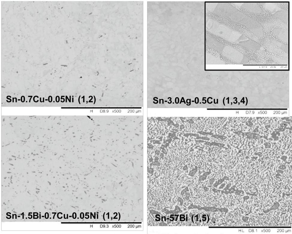
Major Phases Present: 1.  $\beta$ -Sn, 2.  $(\text{Cu,Ni})_6\text{Sn}_5$ , 3.  $\text{Cu}_6\text{Sn}_5$ , 4.  $\text{Ag}_3\text{Sn}$ , 5. Bi
