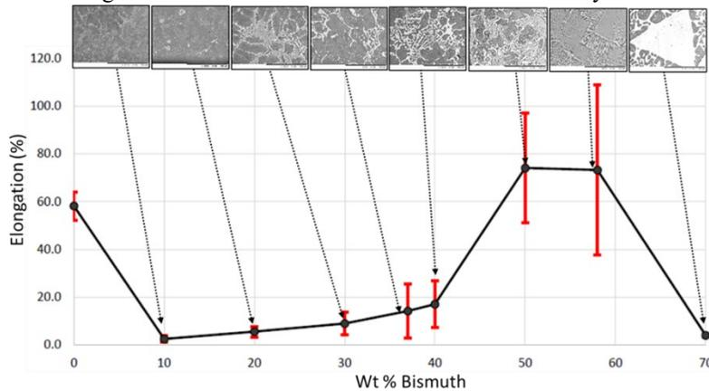
**Figure 15.** Elongation at a strain rate of  $0.00079 \text{ s}^{-1}$  of tin-bismuth alloys as a function of bismuth content.
