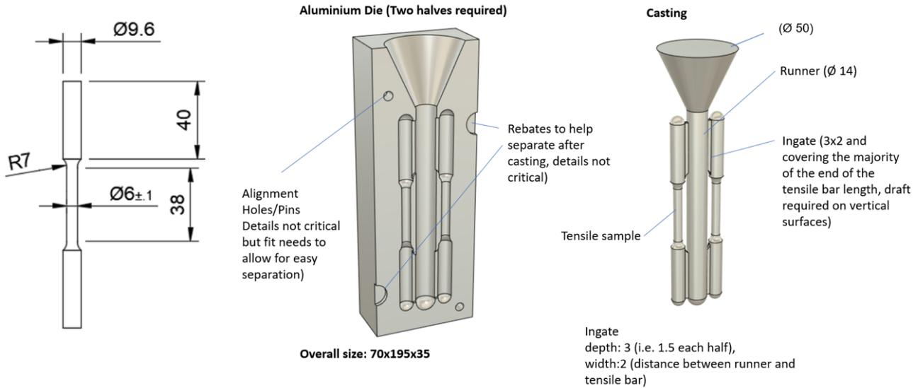
**Figure 2.** Tensile test piece dimensions, mould and casting from which the test pieces were recovered
