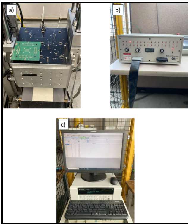
Figure 2. Experimental setup with a.) Lansmont Model 23 Drop table, b.) Anatech event detector and c.) Keysight Data logger
