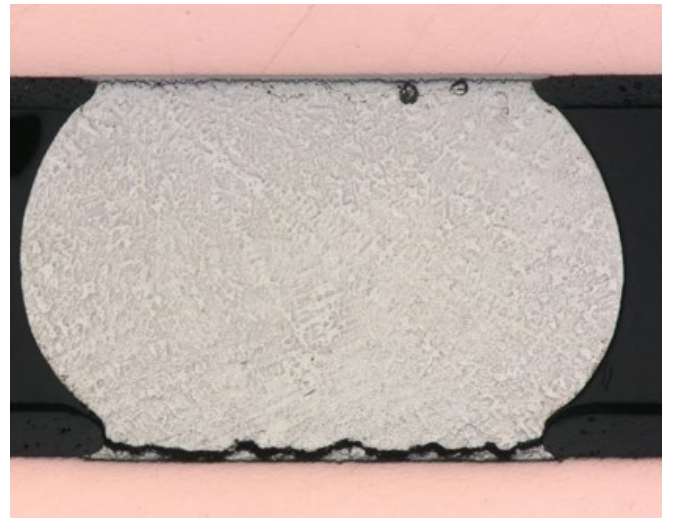
Figure 14. L29 solder joint from the 50 day population. This joint failed at drop #311. Crack growth occurred through the bulk solder above the PCB side IMC region.
