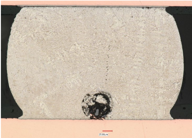
Figure 10. L29 solder joint from the After Reflow population. This joint failed at drop #46. There appears to be a clean separation between the BGA nickel layer and the IMC.
