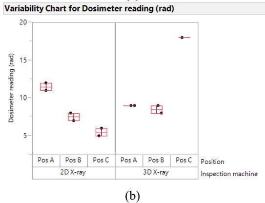
Figure 4. BGA #3 X-ray dosage results. Package is facing away from X-ray source in both machines.
