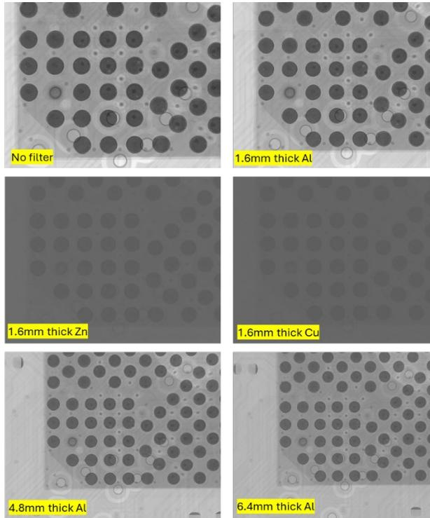
**Figure 6.** 2D X-ray images with various filter materials and thicknesses.
