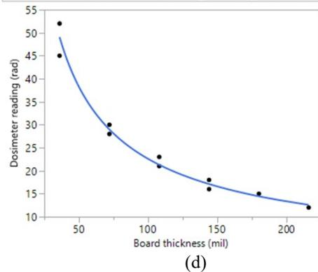
Figure 5. Dependence of dosage on (a) Filter material and thickness, (b) Tool parameters for inspection, (c) Inspection time and (d) Board thickness.
