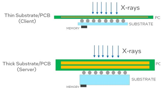
**Figure 8.** Effect of board and substrate geometries on the X-ray dosage absorbed by DRAM.
