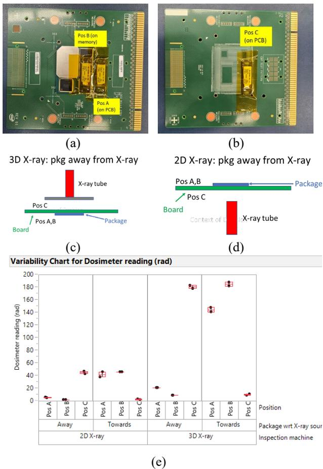
Figure 3. BGA #2 X-ray dosage results.
