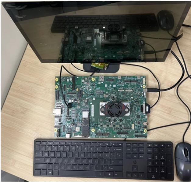
**Figure 1.** Functional test set-up for DRAM performance
