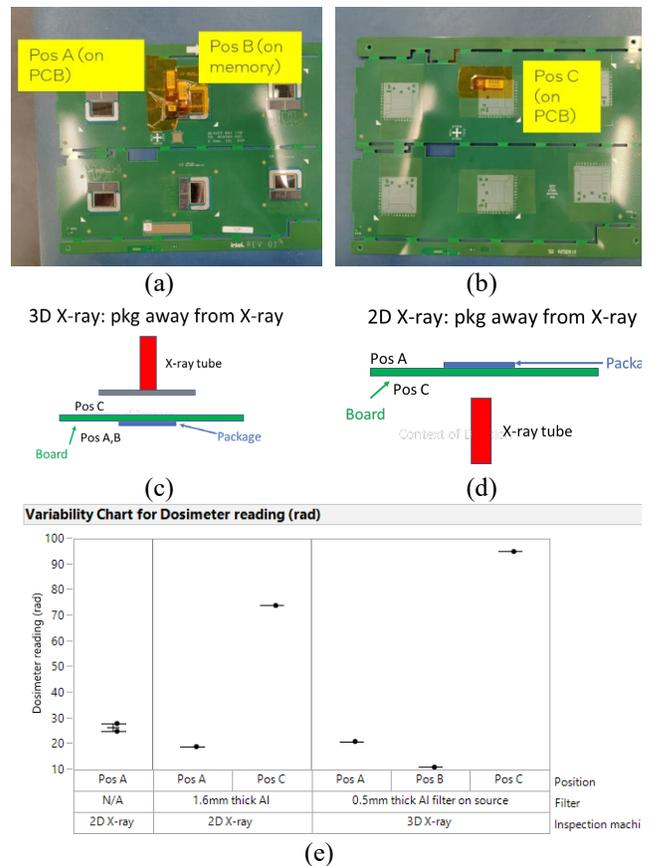
**Figure 2.** BGA #1 results. (a) and (b) Position of dosimeters on the BGA. (c) and (d) Positions of dosimeters with respect to the X-ray source. (e) TLD readings in 2D X-ray (MXI) and 3D X-ray (AXI) machines with different filters.
