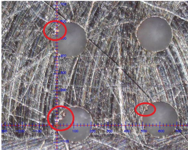
Figure 11. Slag at stencil from Vendor A, Dimension [ \mu\text{m} ]
