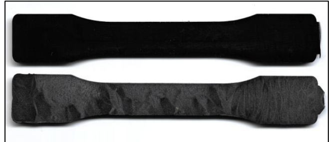
Figure 3: Top test specimen molded with polycarbonate filled with discrete carbon nanotubes and glass flake. Lower test specimen molded with carbon fiber.
