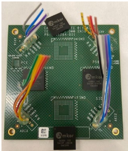
Figure 10. ENIG BGA dummy components were de-attached from board at first drop (for SMD pads). This is a catastrophic solder joint failure.
