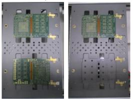
Mirror (Top+Bottom) Top only Figure 3. Support pallet loading card configurations
