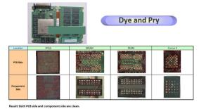
Figure 13. Dye & Pry test result
