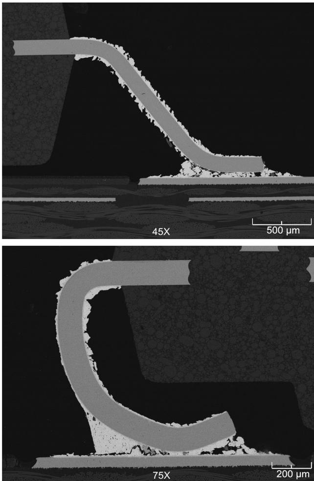
**Figure 16.** SEM images of cross-sections of the gullwing (top) and J-lead (bottom) solder joints of the 172 MaxQFP from Pad D following cycling to failure. Cross-sections were performed at 12,018 board-level -40 to 125°C thermal cycles.
