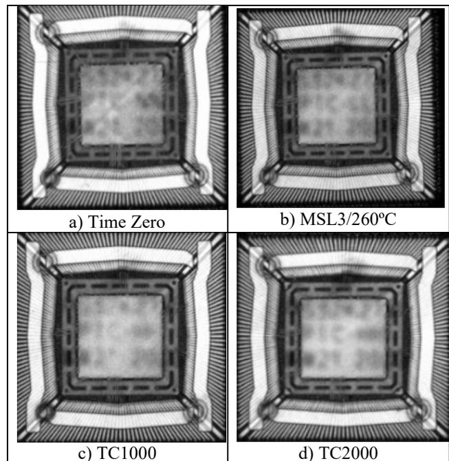
**Figure 7.** C-SAM at time zero and following MSL and temp cycle stressing of the 172 MaxQFP with CMOS40 4ML TV showing no delamination.
