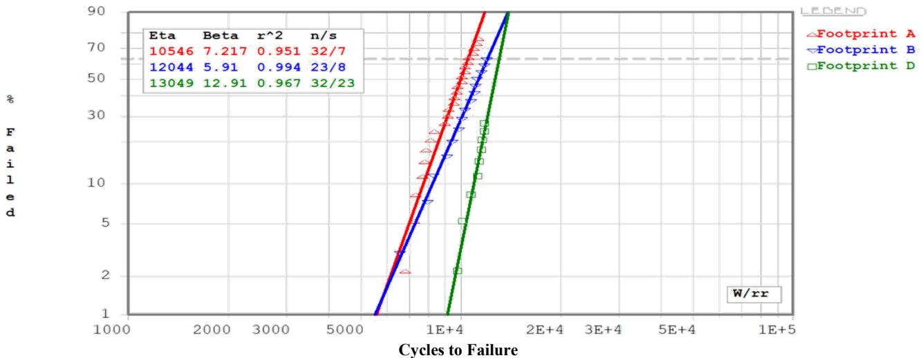
**Figure 15.** Two parameter Weibull plot of board level thermal cycling results for all three PCB pad types.
