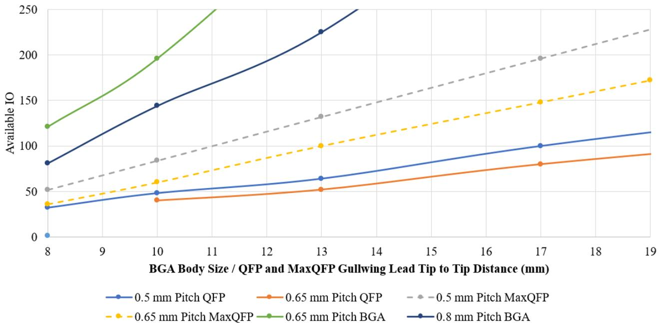
**Figure 6.** IO density comparison between 0.5, 0.65 to 0.8 mm pitch full array BGA and 0.5 and 0.65 mm pitch conventional QFP and MaxQFP. Note that QFP and MaxQFP body size includes the gullwing leads coming out from the package body.
