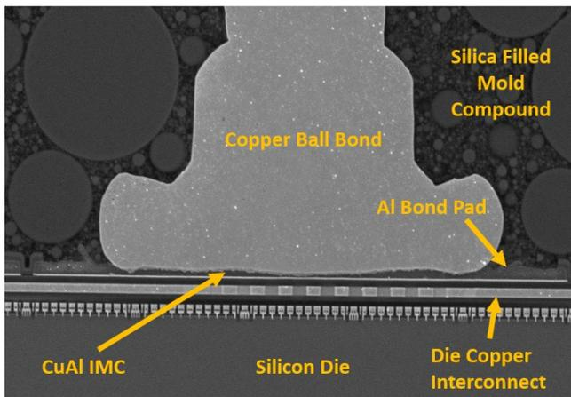
**Figure 8.** Cu ball bond on 172 MaxQFP following TC2000.
