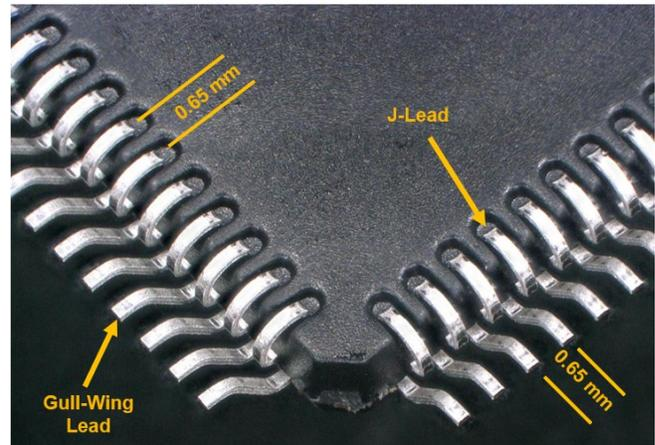
**Figure 2.** Higher magnification of the MaxQFP bottomside showing the interstitially placed J and GW leads.
