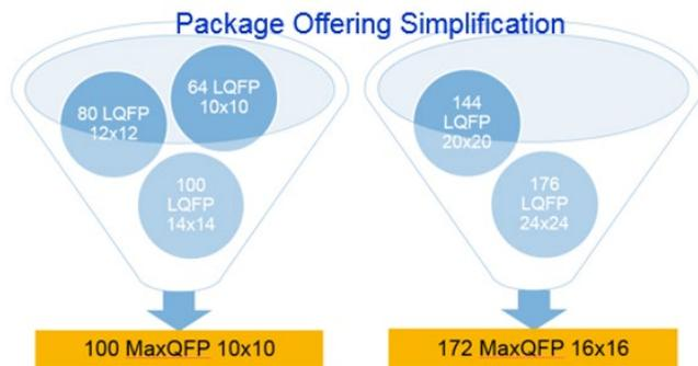
**Figure 4.** MaxQFP simplifies package portfolios as 100 MaxQFP can replace 64, 80 and 100 LQFP, while 172 MaxQFP can replace both 144 and 176 LQFP.
