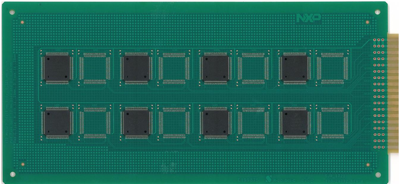
**Figure 9.** Fully assembled 172 MaxQFP test board with all eight type D footprint sites populated. Note edge fingers for in-situ resistance monitoring during thermal cycling.
