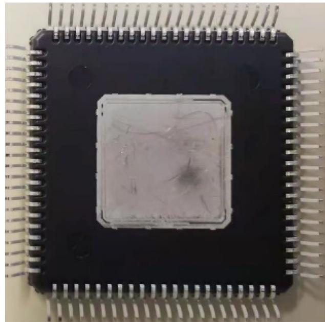
**Figure 5.** Bottomside of the exposed pad version of the MaxQFP slated for more demanding thermal applications.
