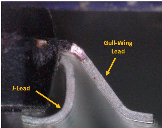
**Figure 3.** MaxQFP package corner showing GW and J-leads.
