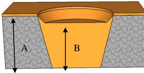
**Figure 4. A typical cross-section of a filled via with a dimple, dimple is the fill difference A-B.**
