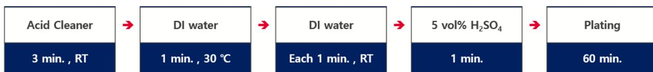
Figure 3. Process flow
