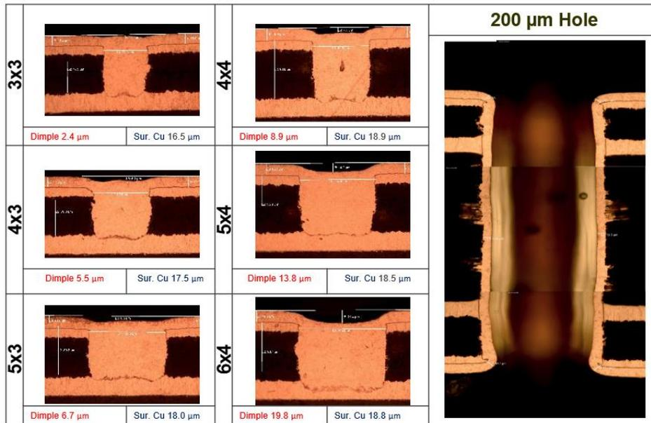
**Figure 8.** Initial viafill and TH plating performance
