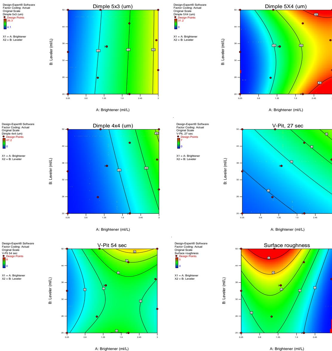
**Figure 9. Surface plots for different interactions of leveler and brightener.**
