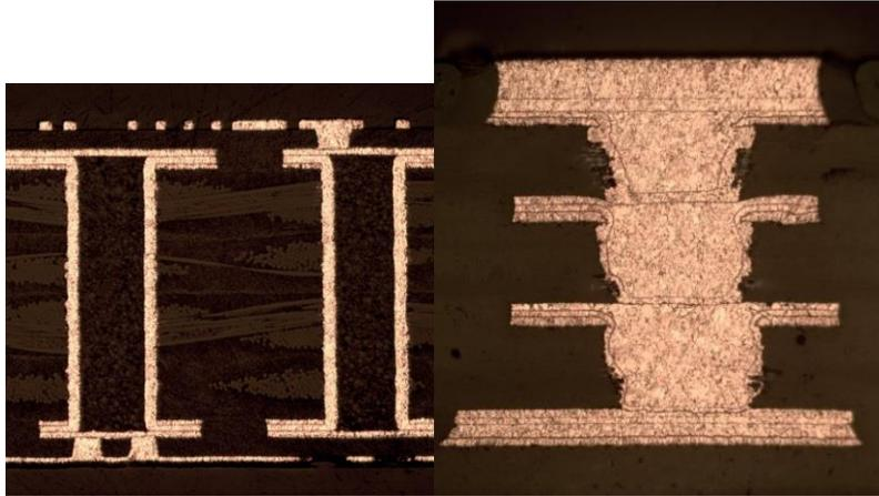
**Figure 1. Multilayer buildup. Several processing layers are visible in the cross-section.**
