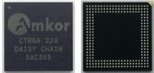
Figure 2. BGA device used in underfill evaluation
