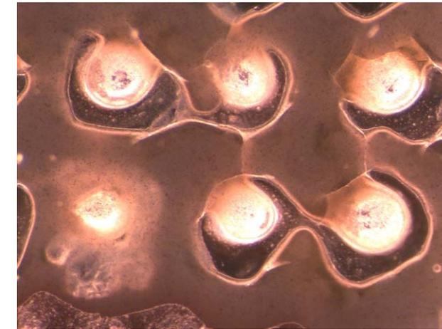
**Figure 19.** Underfill UF-G/Indium 8.9 after 2<sup>nd</sup> reflow
