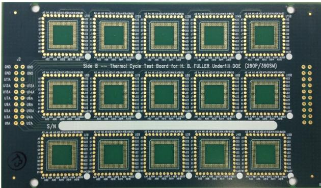
Figure 1. BGA test vehicle for underfill evaluation
