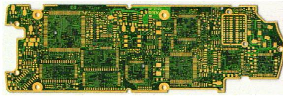
**Figure 3.** Modularized handset motherboard
