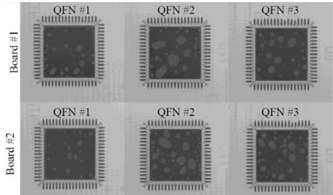
**Figure 6.** QFNs attached with solder paste, no solder fortification preforms used.
