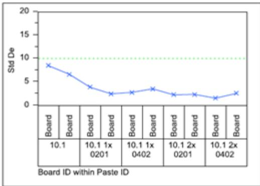
**Figure 14.** Standard deviation of percent voiding in solder joints examined.
