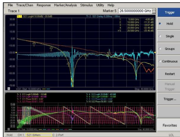
Figure 10 Screen Shot of Single Ended Insertion Loss Testing
