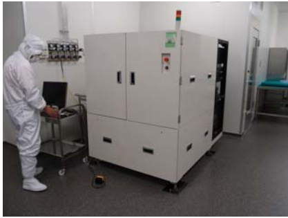
Figure 5. Scanning laser beam induced current (SLBIC) measurement system
