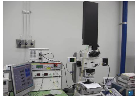
Figure 8. MEMS wafer test system with multimode infrared laser of 1.55 \mu\text{m} in wavelength
