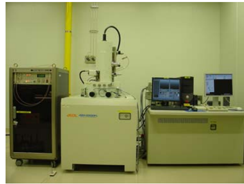
Figure 3. Scanning electron and laser beams induced current (SELBIC) measurement system
