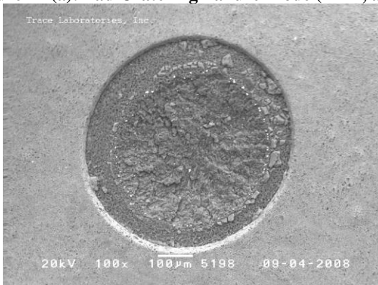
Figure 12 (c): Pad Cratering Failure Mode (HTFP, 6X Reflow)
