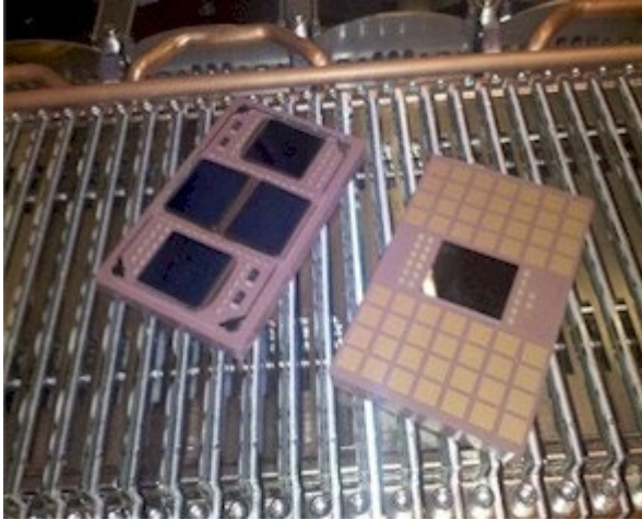
Figure 6. Glass ceramic substrate of CPU and switch-optical transceivers in IBM Power 775.
