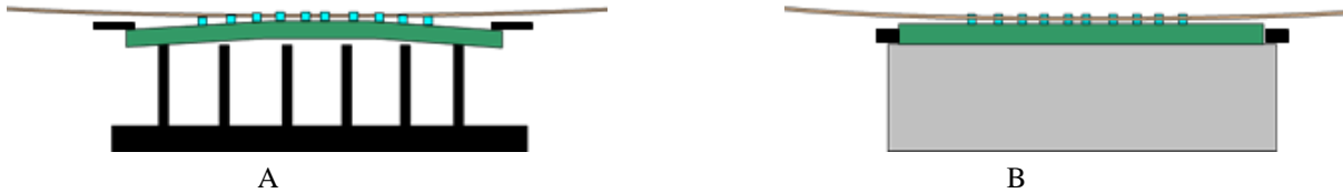
Figure 24 – Illustration of Stencil Separation from PCB A, Support Pin B, Vacuum Support Block
