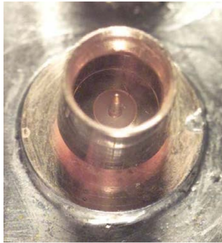
Figure 6. Surface Mount Connector Center Pin Sometimes Failed Mate/Demate.
