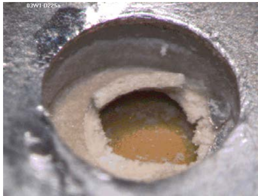
Figure 12. During the Pin Pull Test, the Pin-to-Trace Solder Joint was So Strong that the Trace Pad and the Board Material were Torn Out of the Board.
