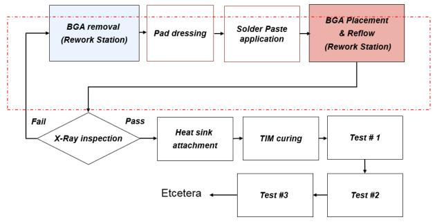
Figure # 1: The BGA rework process:
