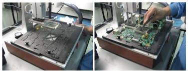
Figure # 23: First prototype of the semi-automated printer
