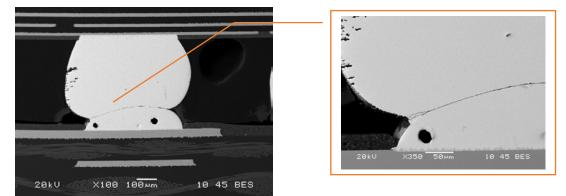
Figure # 8: Cross section SEM image of a "Head in Pillow" found in one of the reworked BGAs
