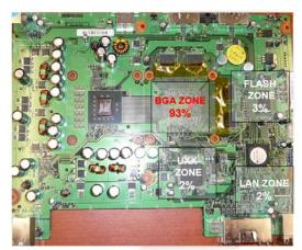
Figure # 2: Defect mapping
