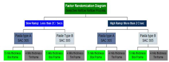
Figure # 13: Example of one of the several DoE's made (Factor Randomization Diagram) to analyze metallurgical incompatibility
