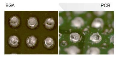
Figure # 11: HiP defect after BGA rip off. Right side is the bottom side of the BGA showing the concavity.
