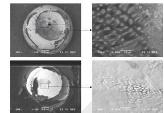
Figure # 12: SEM images of a HiP, no metallurgical incompatibility found, no foreign material found in the EDX analysis.
