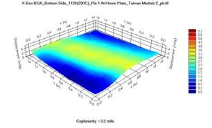
Figure # 15: Thermoiré image of the bottom side of the BGA showing a coplanarity of 3.2 mils along all BGA Ball at 230°C
