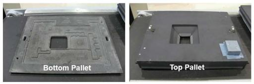
Figure # 6: Reflow protective fixture
