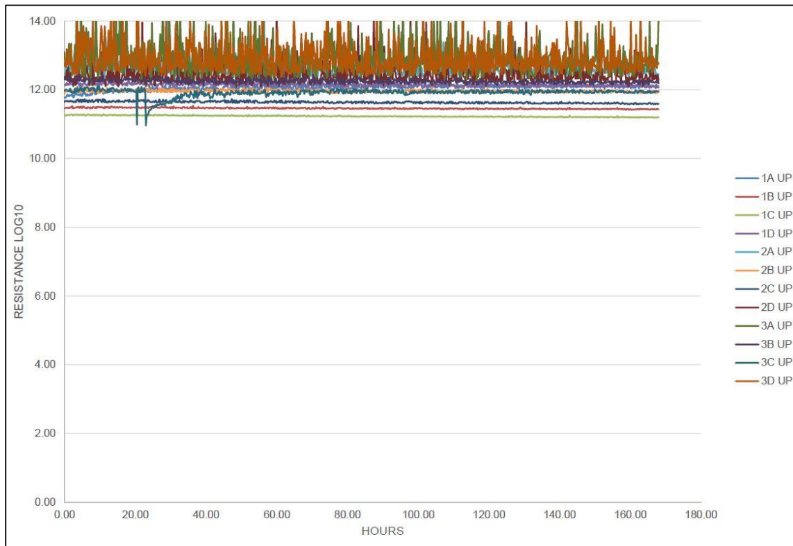
Figure 7. Flux C, (Rosin-Containing) Pattern Up SIR Results
