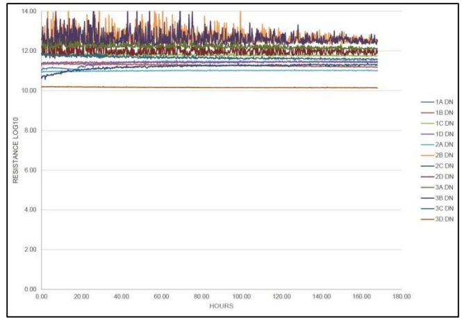
Figure 8. Flux C, (Rosin-Containing) Pattern Down SIR Results
