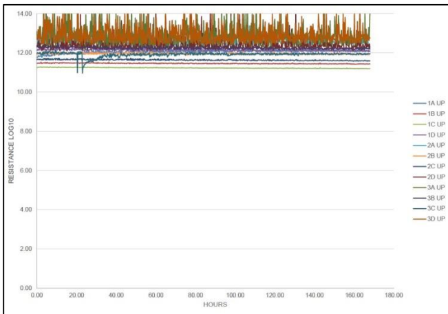
Figure 7. Flux C, (Rosin-Containing) Pattern Up SIR Results
