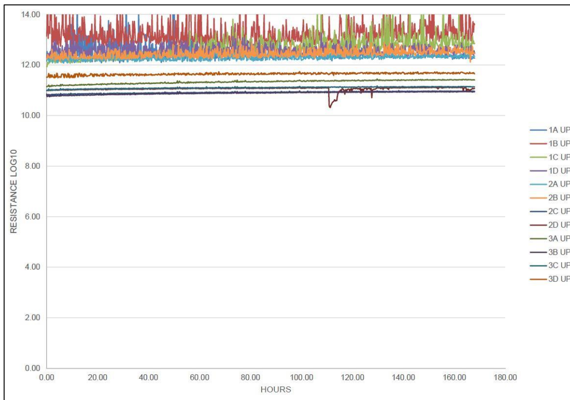
Figure 5. Flux B, (Rosin-Containing) Pattern Up SIR Results
