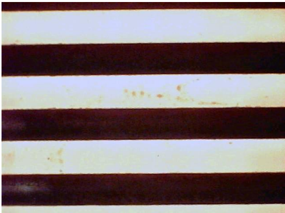
Figure 17. Example of a Failing SIR Board Backlight 30X Mag
