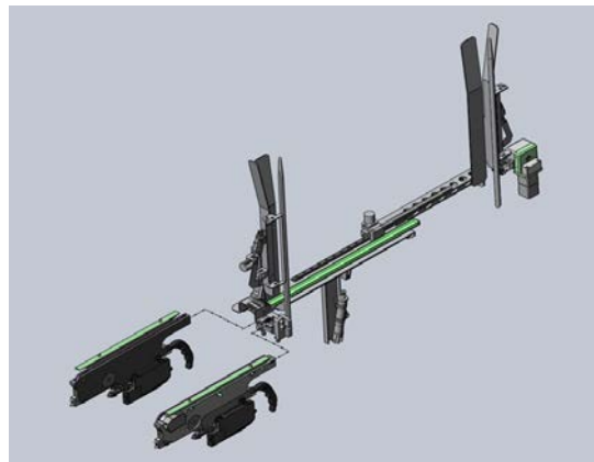
Figure 9 - Adjustable Stack tube feeder
