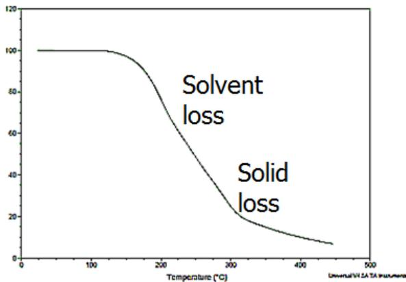
**Figure 3.** Flux vaporization behavior [1]
