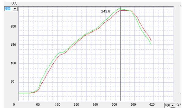
**Figure 9.** Reflow profile used for fluxed SIR boards with or without glass slides attached.
