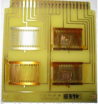
**Figure 8.** Example of reflowed SIR board with glass slide, with 3 comb patterns printed with flux, and 2 of these 3 comb patterns were further covered with glass slides.
