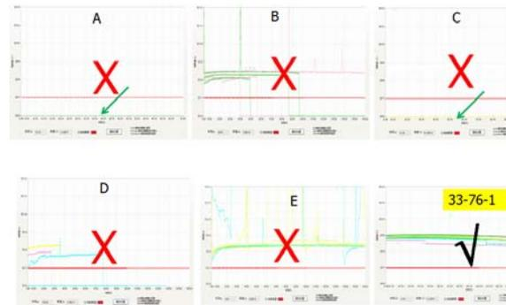
**Figure 15.** SIR data with glass slide on of various fluxes shown in Table 1.
