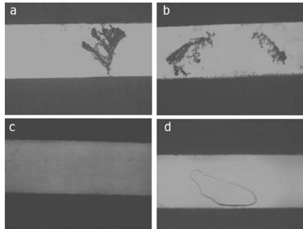
**Figure 16.** Close up look of SIR coupons after SIR test with glass slide on (50X), with a, b showing dendrites, and c, d free of dendrites.
