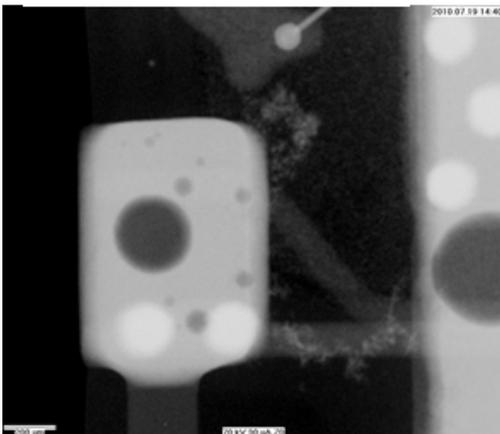
**Figure 6.** Dendrite formation around the large pad of a bottom-terminated component
