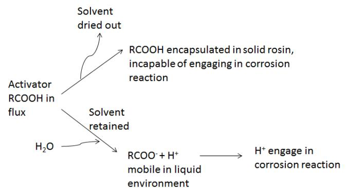
**Figure 5.** Activator RCOOH behavior under different process condition
