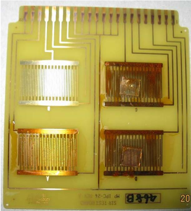
**Figure 8.** Example of reflowed SIR board with glass slide, with 3 comb patterns printed with flux, and 2 of these 3 comb patterns were further covered with glass slides.
