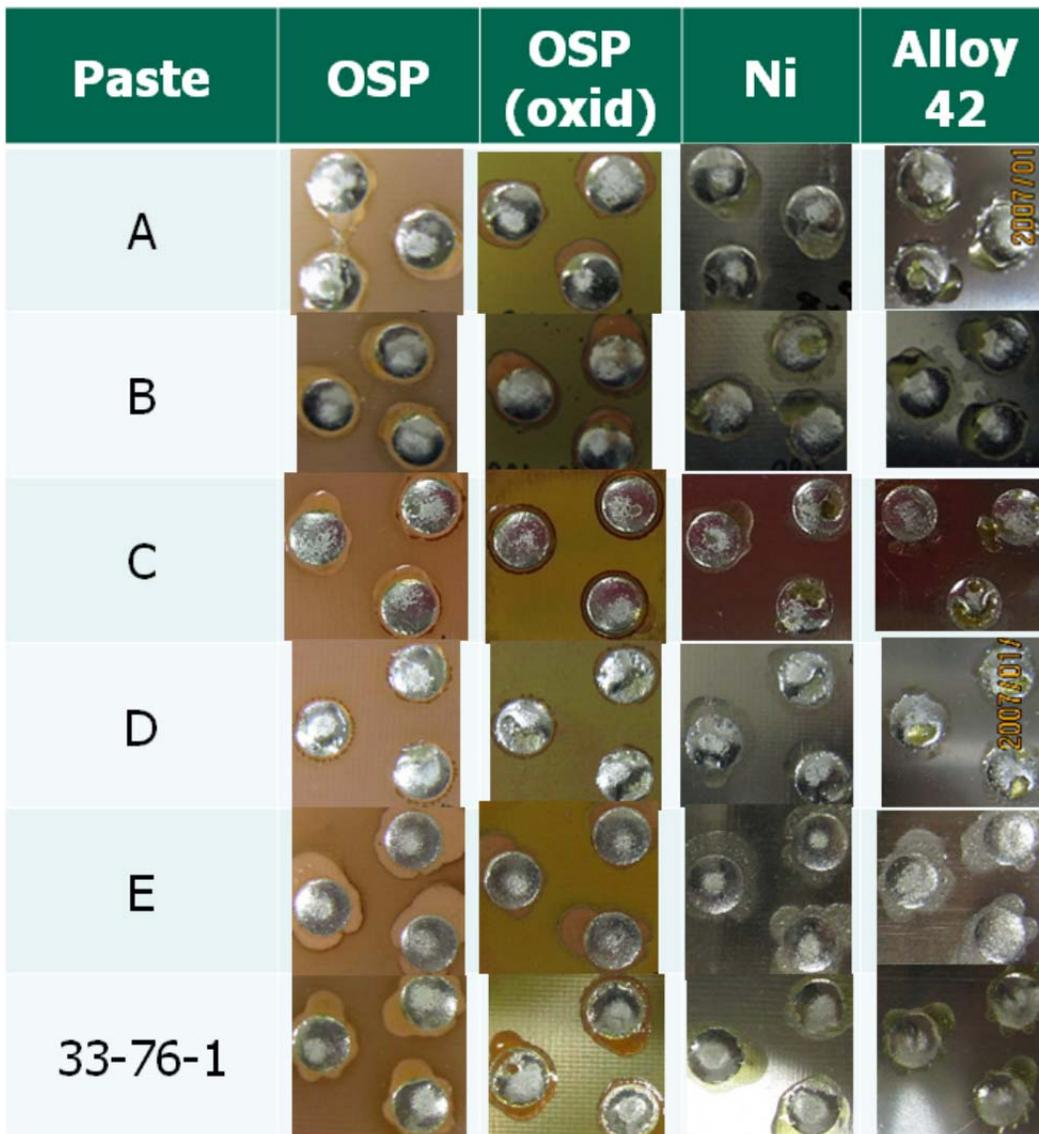
Figure 17. Wetting of solder pastes under air on various substrates.
