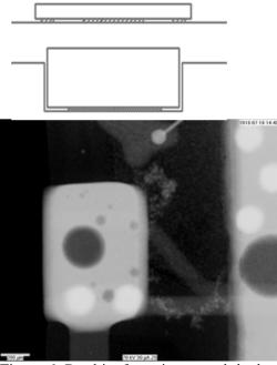
**Figure 6.** Dendrite formation around the large pad of a bottom-terminated component
