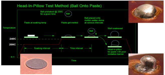
Figure 13. Ball Onto Paste method for HIP propensity evaluation.
