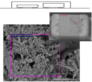
**Figure 7.** Dendrite formations for chip capacitor covered by an electromagnetic shield without venting hole
