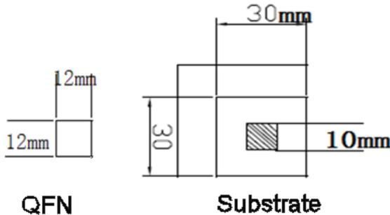
**Figure 11.** Schematic drawing of QFN coupon and substrate.
