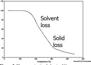
Figure 3. Flux vaporization behavior [1]
