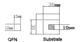
Figure 11. Schematic drawing of QFN coupon and substrate.
