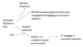
**Figure 5.** Activator RCOOH behavior under different process condition
