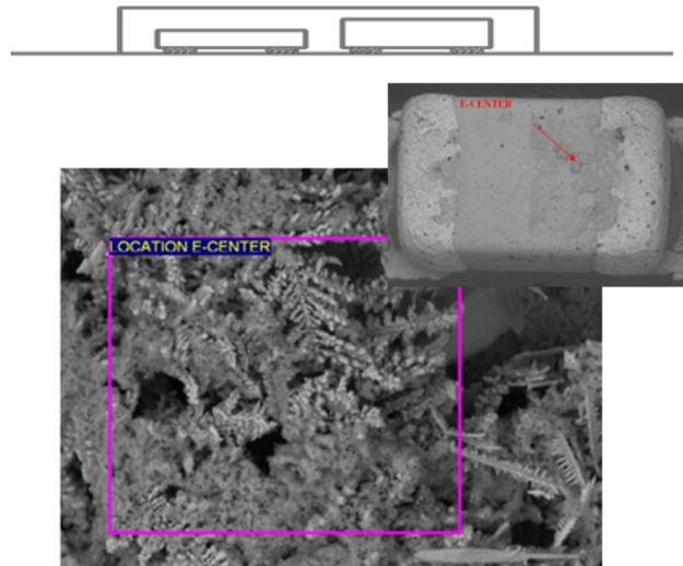
**Figure 7.** Dendrite formations for chip capacitor covered by an electromagnetic shield without venting hole
