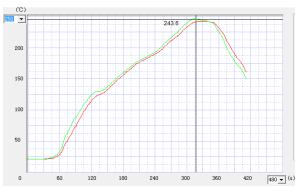
**Figure 9.** Reflow profile used for fluxed SIR boards with or withou glass slides attached.
