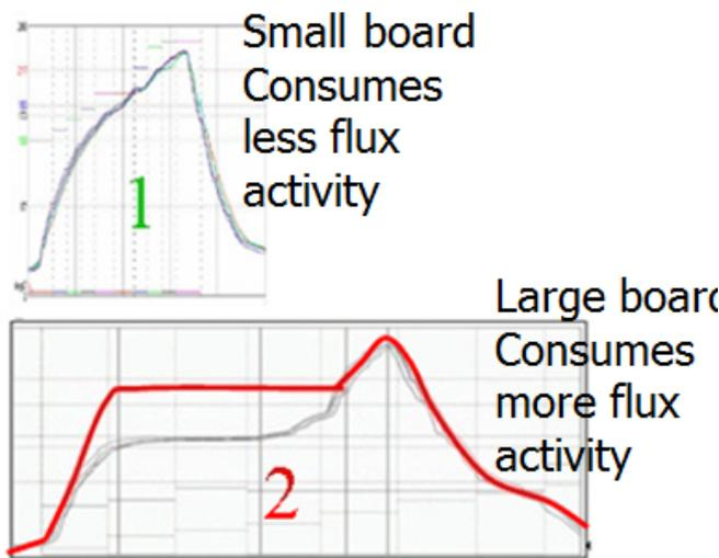
**Figure 4.** Flux activity consumption varies with profile type [2]
