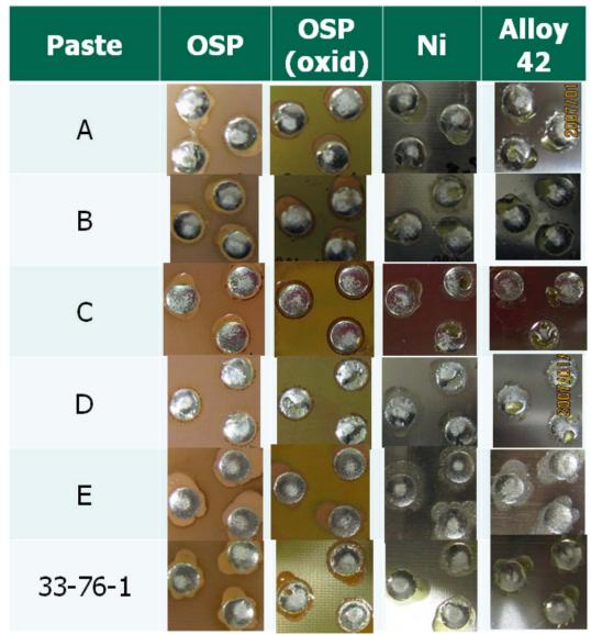
Figure 17. Wetting of solder pastes under air on various substrates.
