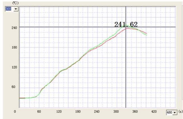
**Figure 12.** Reflow profile used for QFN voiding test.
