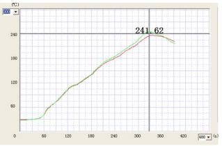
Figure 12. Reflow profile used for QFN voiding test.
