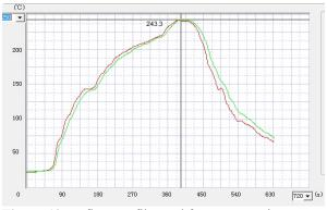
Figure 10. Reflow profile used for paste wetting test.
