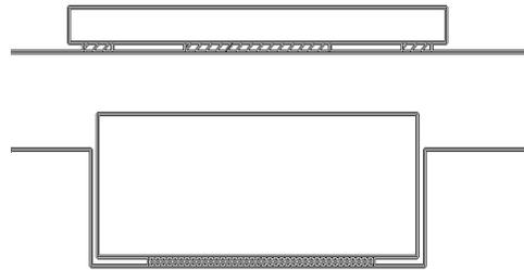
**Figure 1.** Schematic drawing of low standoff components and components assembled in the cavity of substrate.
