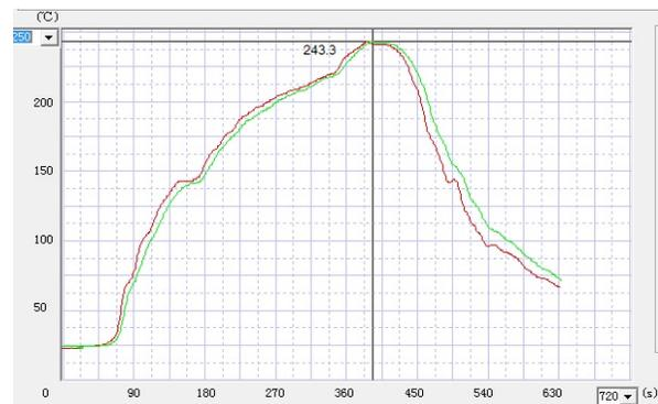
**Figure 10.** Reflow profile used for paste wetting test.
