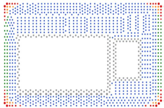
Figure 5 Different colors depict different solder volumes on the same package
