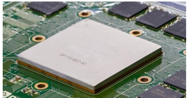
Figure 3 BGA with integral heat sink
