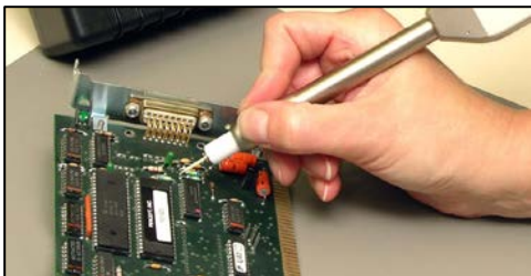
Figure 4. Measuring PC conductor with high an impedance contact volt meter
