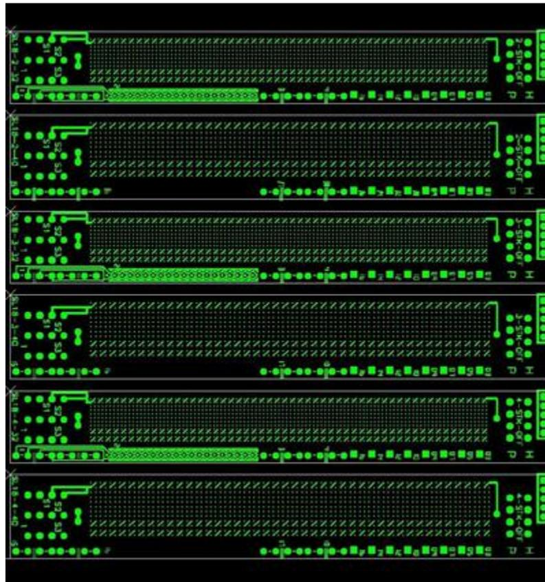
**Fig.3: Sub-Panel Coupon Layout**
