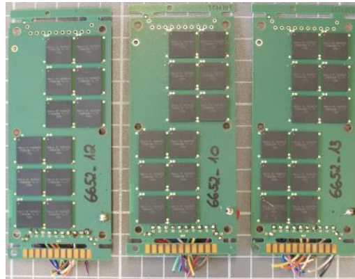
Figure 10: Assembled coupons (TV1) for thermo cycle testing
