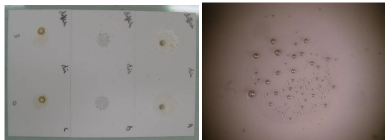
Figure 13. c) A, B, C without preheat after 4 h ambient temperature d) Explosion
