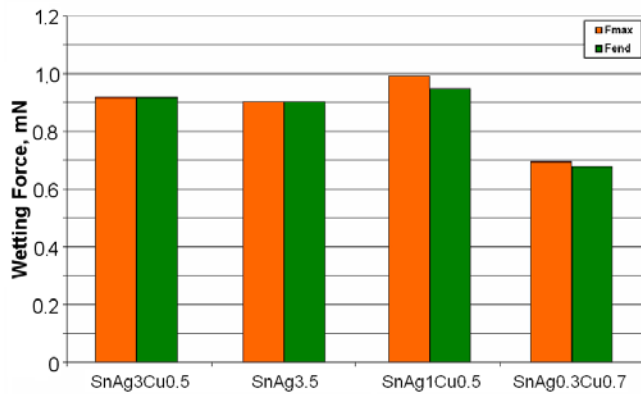
Figure 6. Evaluation of average wetting forces, tested with the solder globule method at 235°C
