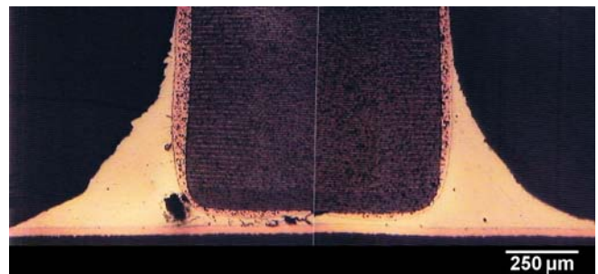
Figure 13. Cross section of a SnAg0.3Cu0.7 solder joint of a CC1206 component after 1000 cycles
