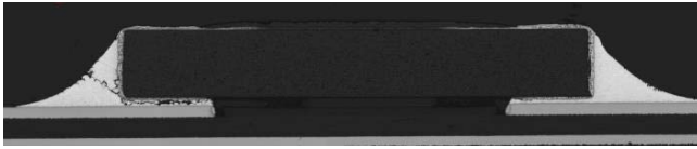
Figure 3a. Cross section for Chip 1206, SAC, N=6500 field cycles 22/93 (4 ½ years) [3]
