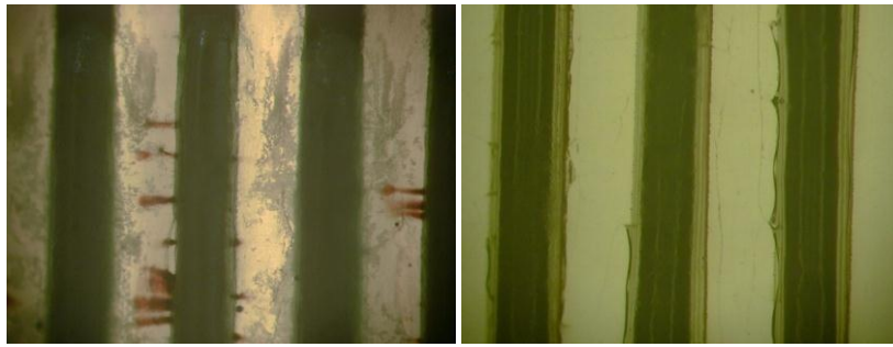
Figure 9. Observation under back-light a) Dendrites with paste C, b) No dendrite with paste D
