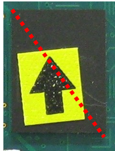
Figure 1 The BGA component with the red dotted line indicating the cross section area.
