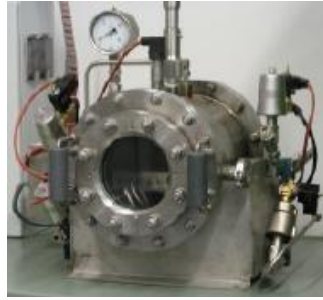
Figure 9 – Laboratory setup of pressure container with controlled heating
