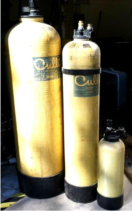
Photo 1 Fiberglass absorptive media tanks
