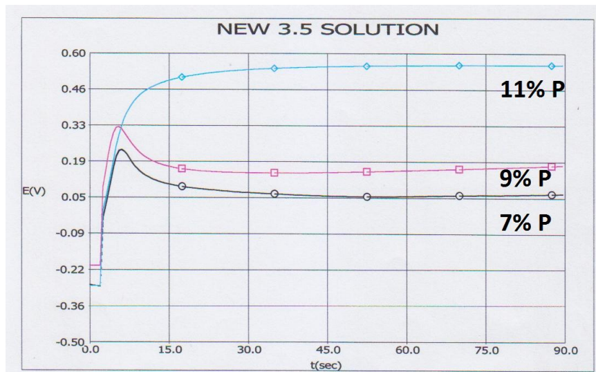
Figure 3. SERA corrosion test comparing 7, 9 and 11 wt. %P EN surfaces with 2 M KCl,
