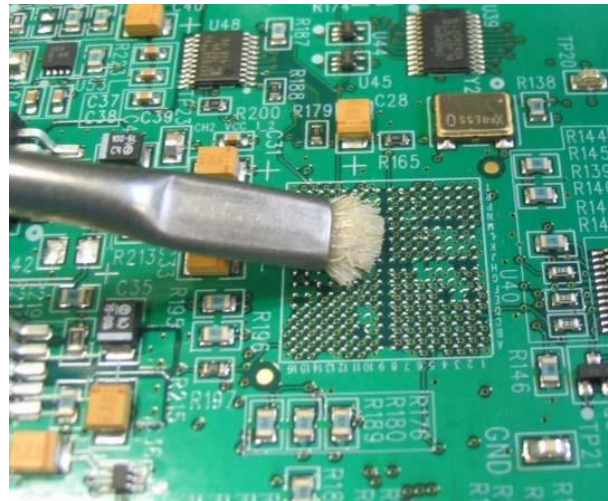
Figure 4. Gel flux application on pads using a brush
