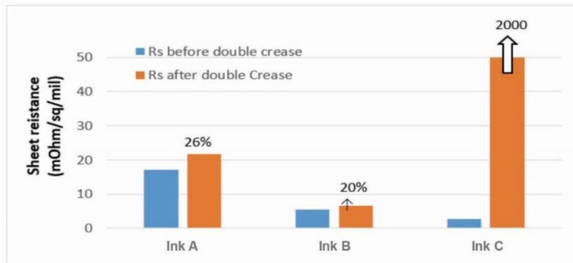
Figure 6: Sheet resistance before and after double crease test
