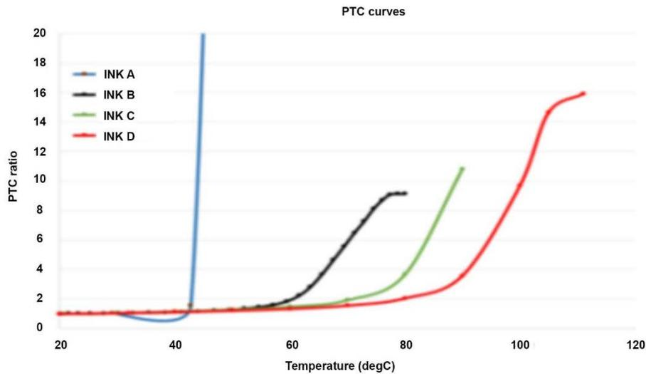
Figure 12: Plot of PTC ink maximum temperature curves
