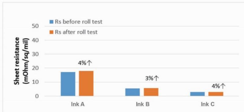
Figure 5: Sheet resistance of silver conductive inks before and after roll test
