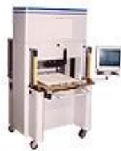
Figure 16. Servo Electric Press 12 tons
